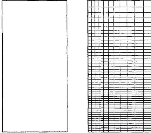
Figure 1: Initial configuration for a fractured material degradation with the 686 Finite Element mesh.
