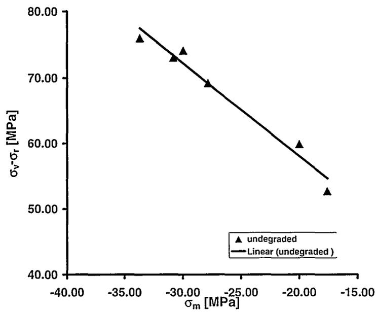
Figure 6: Undegraded paste in deviator-mean stress plane
