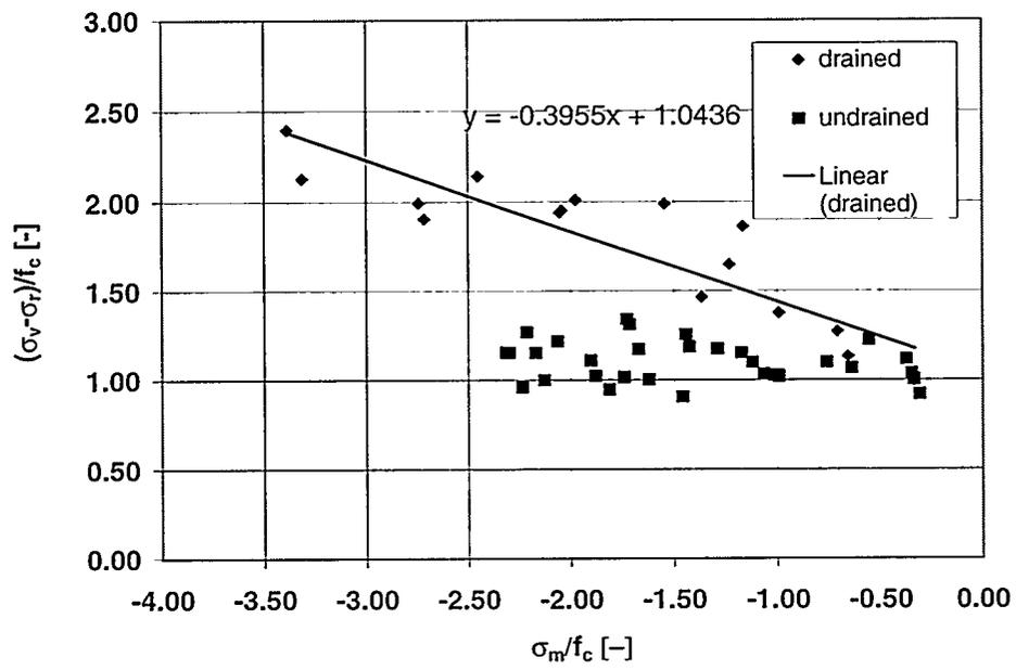
Figure 7: Degraded paste in deviator-mean stress plane (Drained and undrained)
