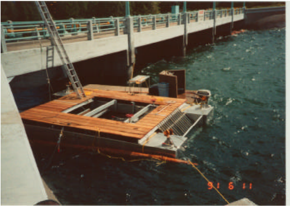
Figure 10. Floating smolt bypass trap above radial gates at spillway of Cle Elum dam.
