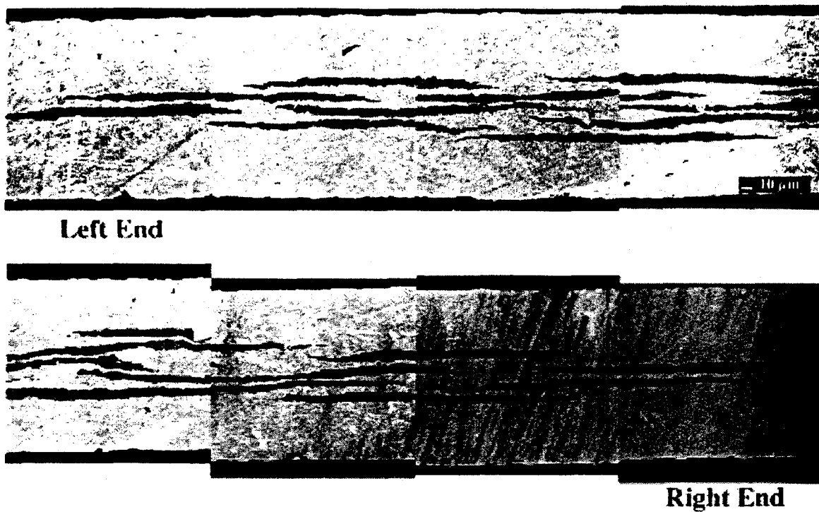
Fig. 8. Transverse section of a Bi-2223 composite specimen subjected to an optimized thermal-slide heat treatment.
