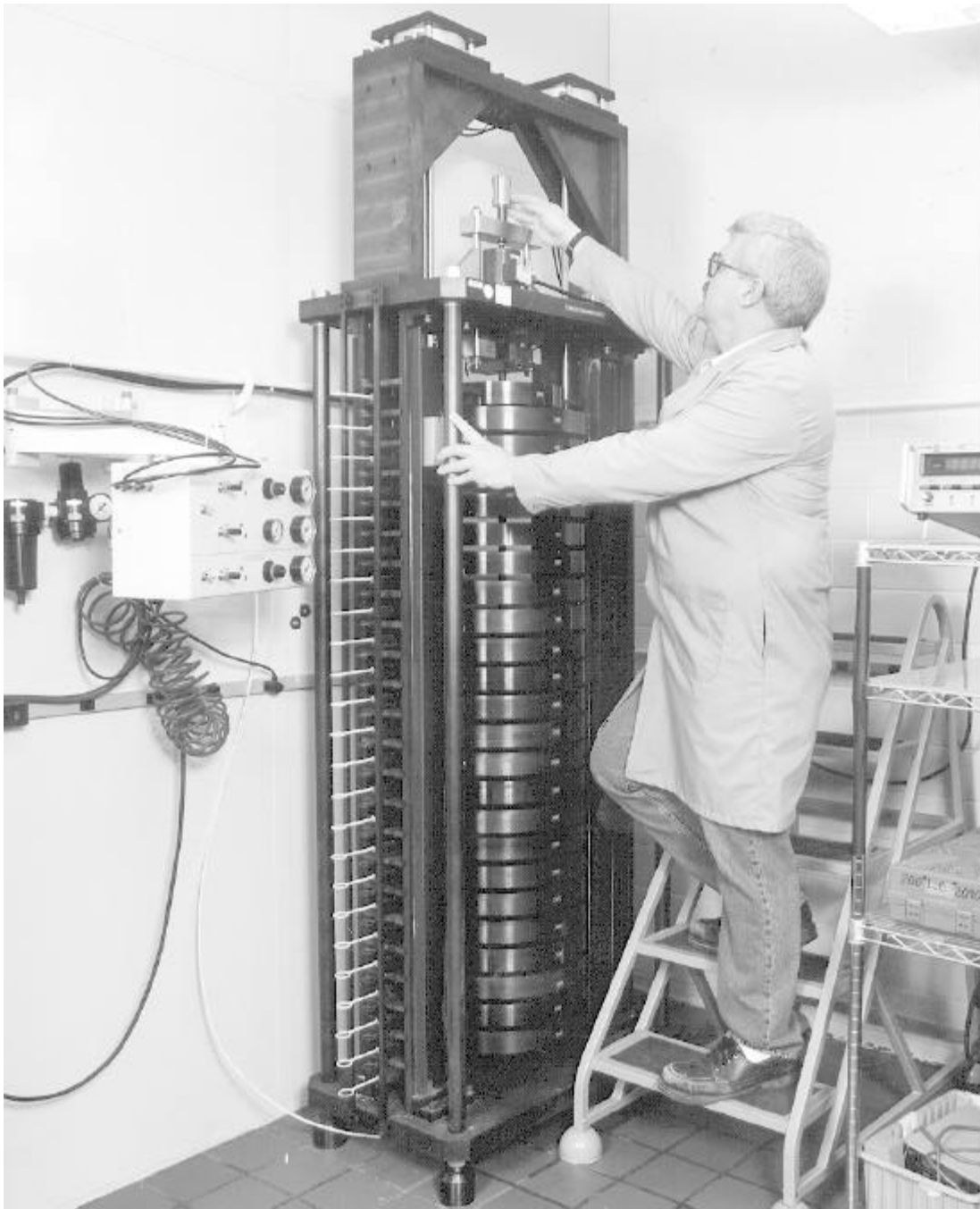
Dead Weight Force Calibration
