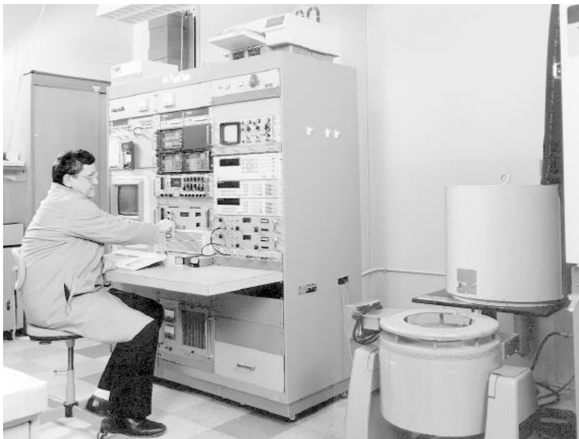
Accelerometer Vibration Calibration
