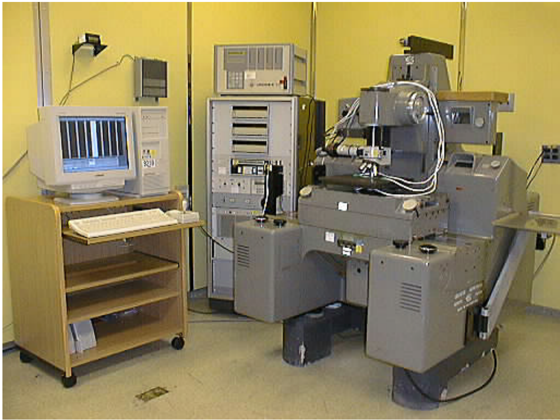
CMM With Video Edge Detection System
