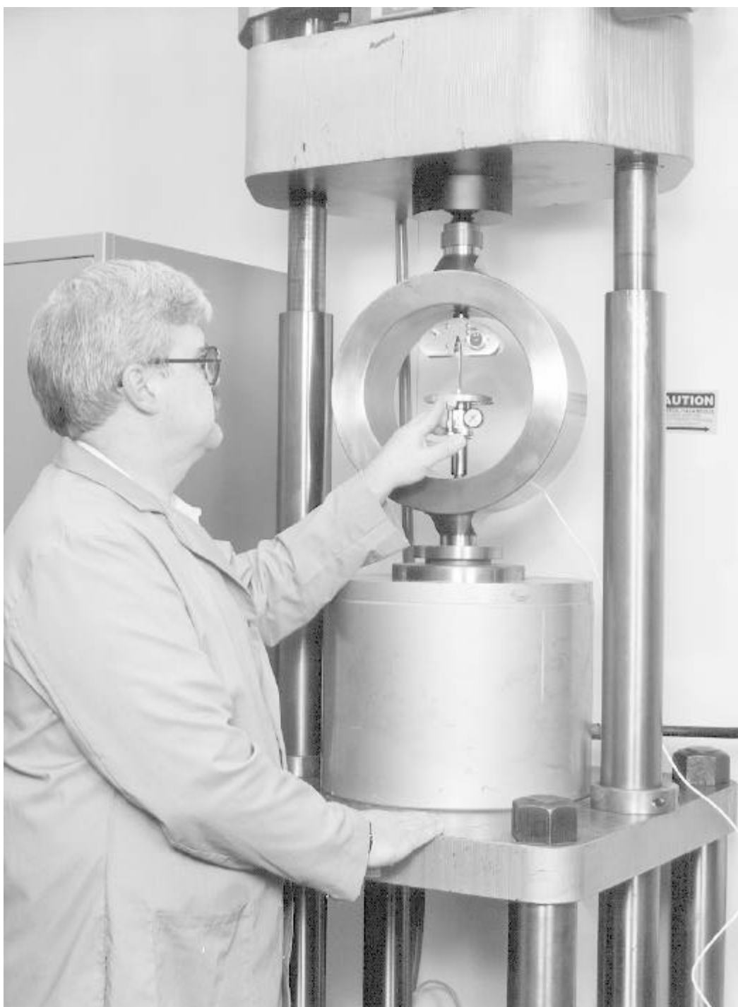
Proving Ring Calibration
