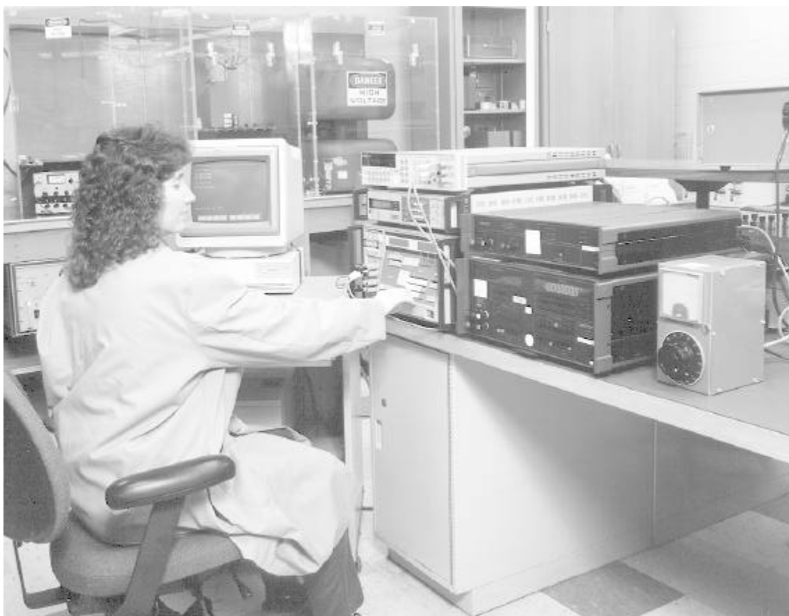
Automated Digital Multimeter Calibration
