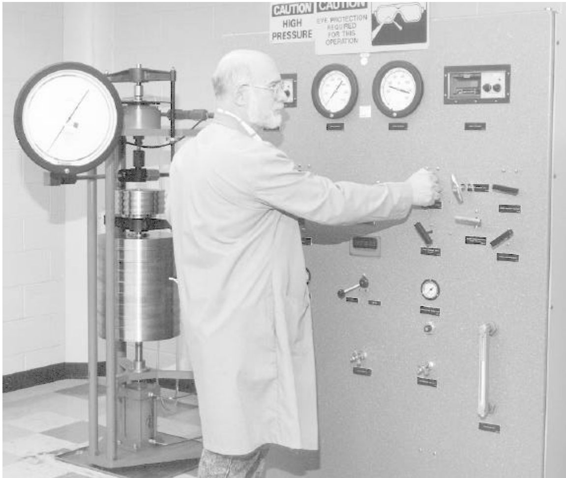
Pressure Calibration Using Controlled Clearance Dead Weight Piston Gage
