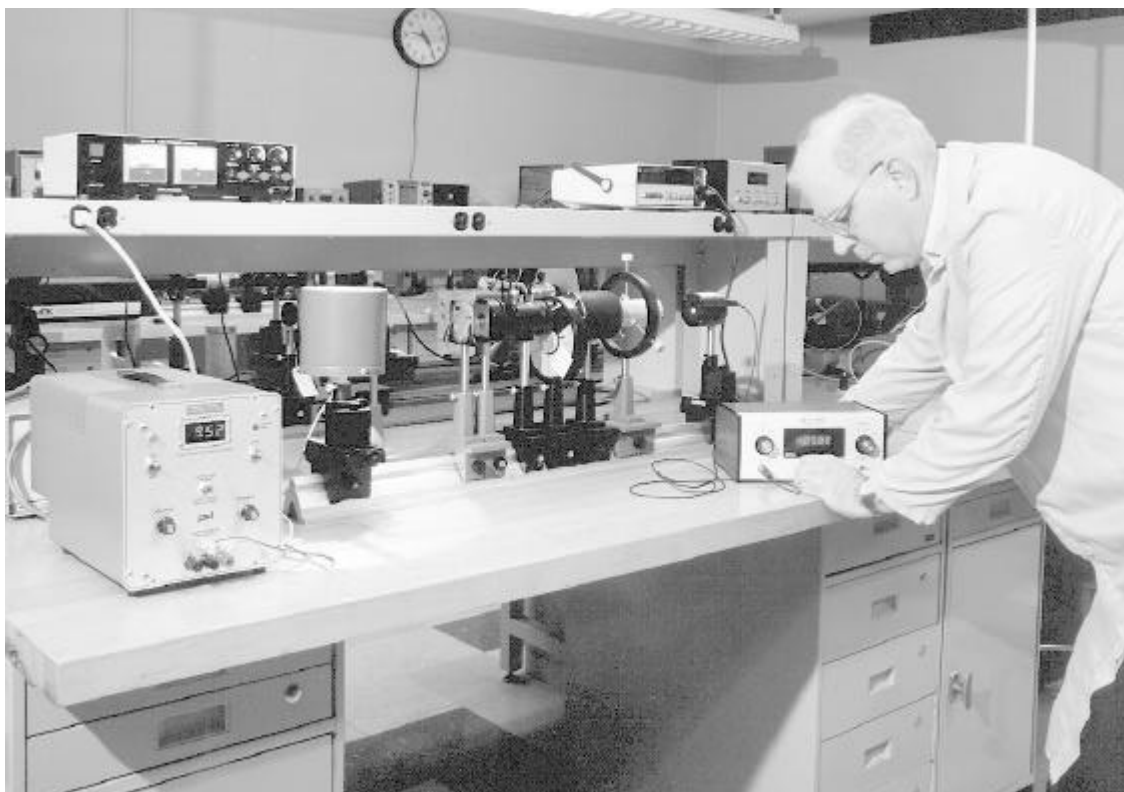
Photodiode Detector Calibration
