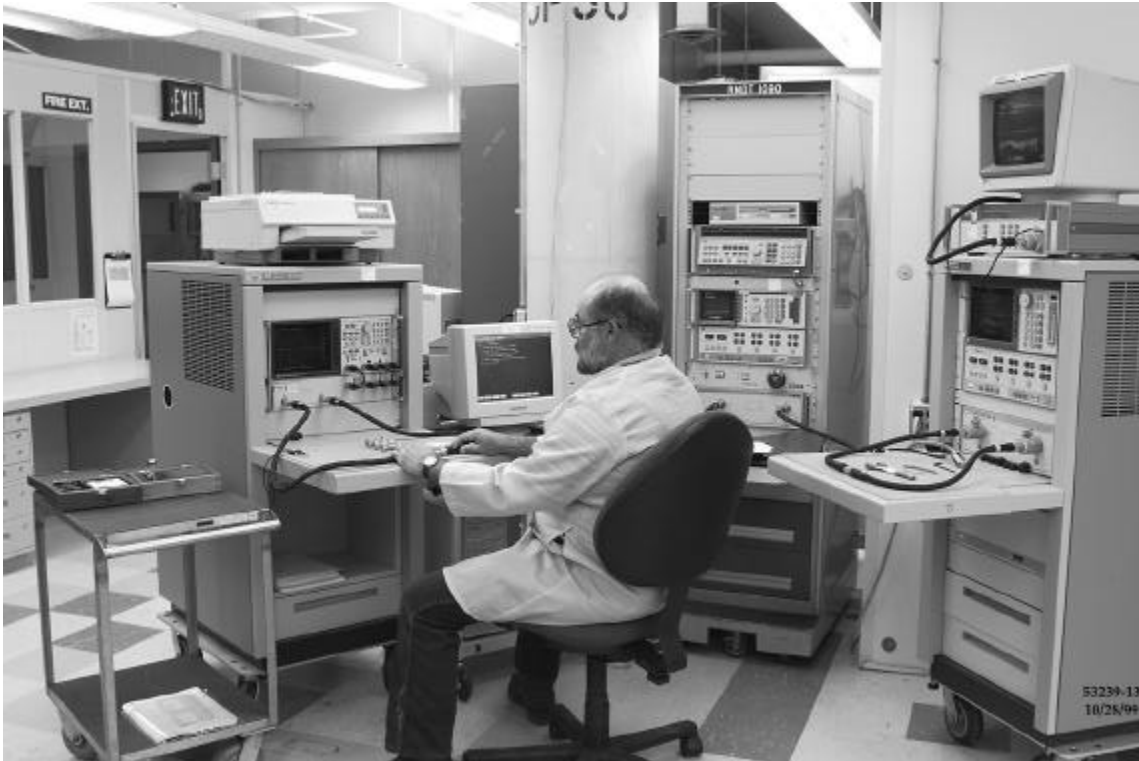
Attenuator Calibration Using an Automatic Network Analyzer
