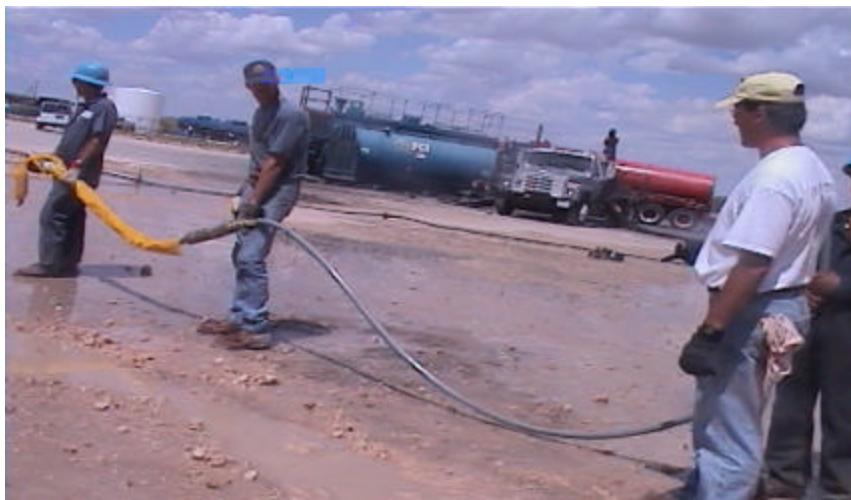
Fig. 12. Series of photographs showing the MPI floor tool being activated at surface: (a) overview of turbulence created by MPI vertical and floor tools, (b) close-up of MPI floor tool, (c) tool and hose after 5 min of jetting at 400 gpm and 6,000 psi. Note: All information in this Figure is marked as limited rights data under the terms of the subcontracts between GES and LMER. MPI is protected under U.S. Patents Nos. 5,860,907 and 5,645,377 with several other patents pending.
