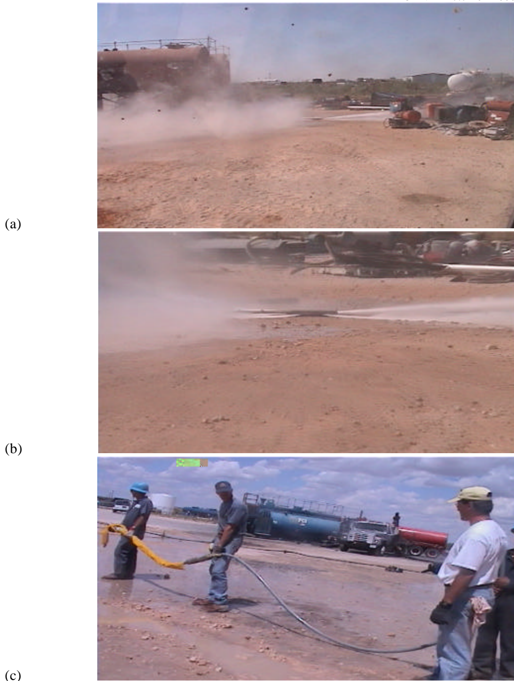
Fig. 6. Series of photographs showing MPI floor tool being activated at surface: (a) overall view, (b) close-up of MPI jetting tool, and (c) tool and hose after 5 min of jetting at 400 gal/min and 6,000 psi. Note: All information in this Figure is marked as limited rights data under the terms of the subcontracts between Ground Environmental Services and Lockheed Martin Energy Research. MPI is protected under U. S. Patents Nos. 5,860,907 and 5,645,377 with several other patents pending.
