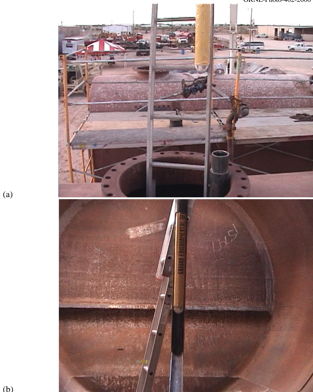
Fig. 4. Close-up photographs of MPI tool: (a) Insertion into 4-in.-diam riser pipe and (b) lowering through carrier casing inside SRS tank. Note: All information in this Figure is marked as limited rights data under the terms of the subcontracts between Ground Environmental Services and Lockheed Martin Energy Research. MPI is protected under U. S. Patents Nos. 5,860,907 and 5,645,377 with several other patents pending.
