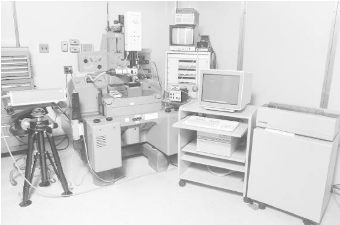
Figure 1. SIP Trioptic CMM With Laser-Based Edge Detector
