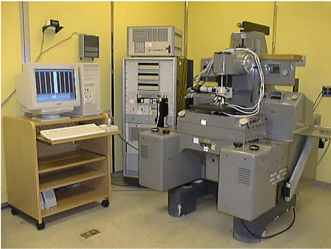
Figure 3. Trioptic With New Vision System
