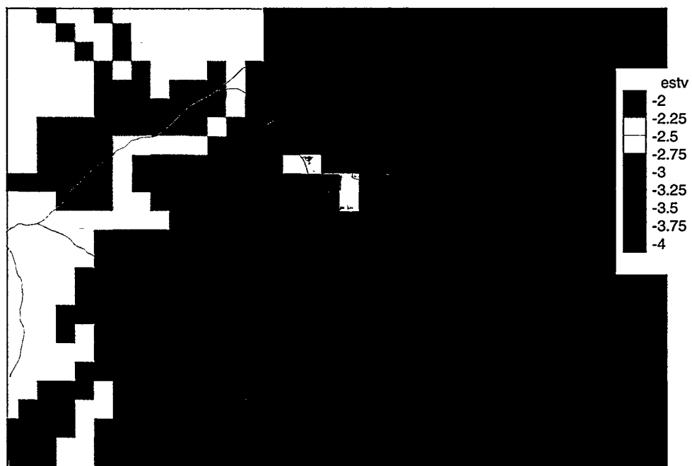
Figure G-23. Kriging estimates for Kv in model layer 6 (~TZ); before TCCZ mods.
