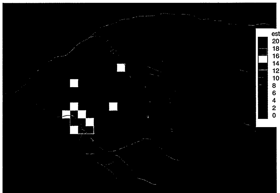
Figure G-22. Kriging estimates for Kh in model layer 6 (~TZ); before TCCZ mods.
