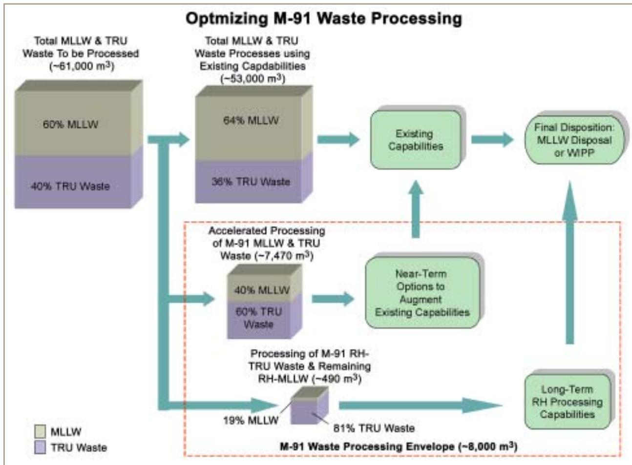
Figure S.1. M-91 Waste Conceptual Processing Flow Diagram
