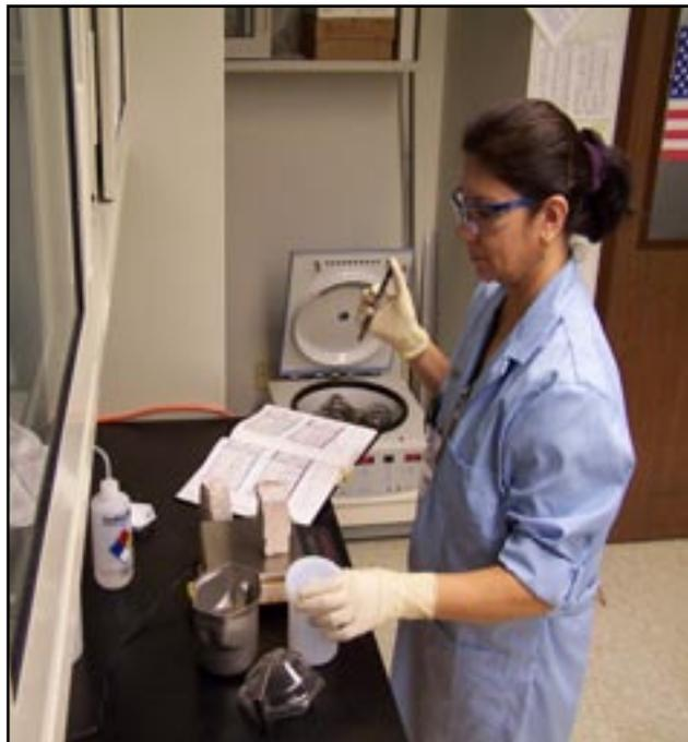
*A PNNL researcher prepares to use a centrifugation technique to remove the pore-water extractable rhenium from castable refractory samples. Rhenium is a non radioactive surrogate for technetium in laboratory studies.*
