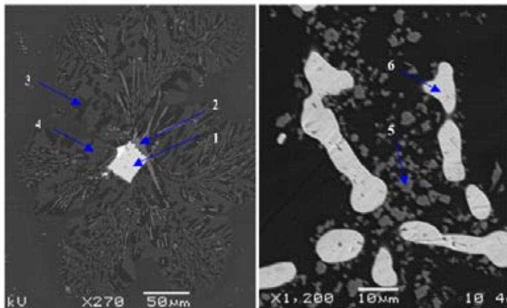
*Crystalline phases were identified in AMP1-03-SC glass (1-Baddeleyite; 2-Sodium-zirconium silicate; 3-nepheline; 4-combeite, 5-spinel, 6-Fe metal) using a scanning electron microscope.*
