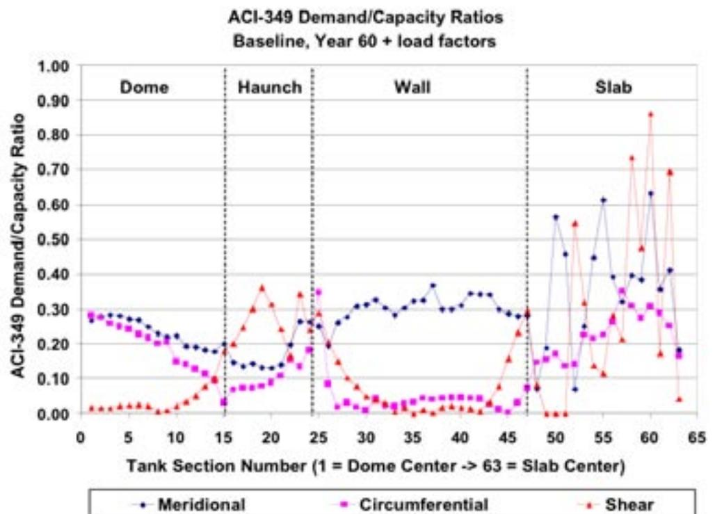
*A typical analytical result for the concrete shows the demand/capacity ratio at each cross section of the tank.*
