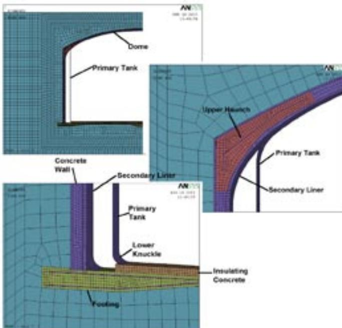
*Using a computer modeling software, PNNL analyzed the thermal and operating loads for Hanford's double-shell tanks.*
