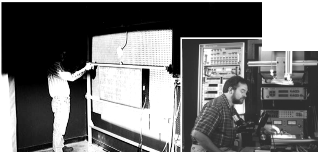
Fig. 2.1. Large (left) and small (right) scale solar simulators for evaluating PV performance in the laboratory.
