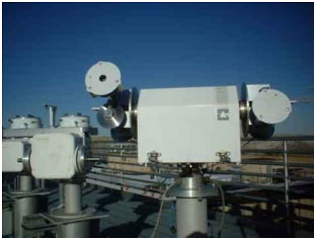
Fig 3.16. Photo of pyrheliometers with window (lower left), window and flange (right), and flange only (top left) shaded.
