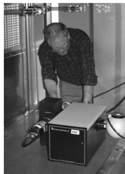
Fig 2.2 Scanning grating monochromator with integrating sphere input optic.
