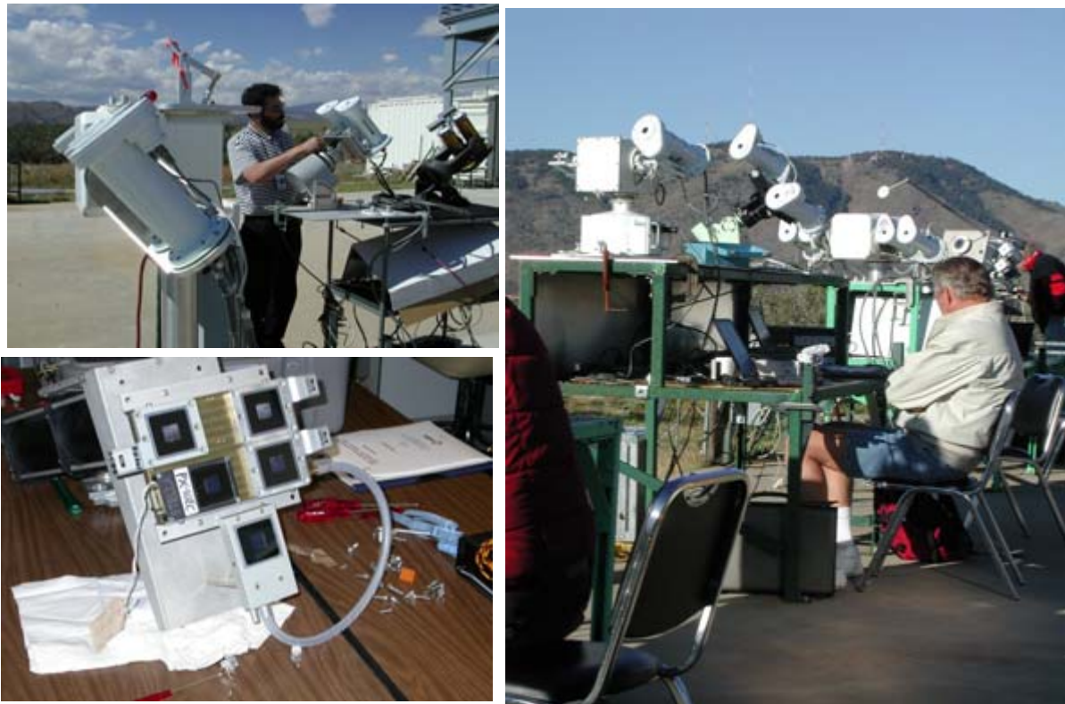
Fig. 3.4. NREL Pyrheliometer Comparison (NPC) September 23-October 3, 2004. Top Left; NREL Metrologist I. Reda adjusts the NREL reference group of absolute cavity radiometers. Bottom left, European Solar Testing Institute (ESTI) PV Reference Cell packages tested during the comparison. Right, subset of the 17 absolute cavity radiometers participating in the NPC, including representatives from National Oceanic and Atmospheric Administration, National Aeronautics and Space Administration, Sandia National Laboratories, ESTI, and instrument manufacturer Eppley Laboratory.
