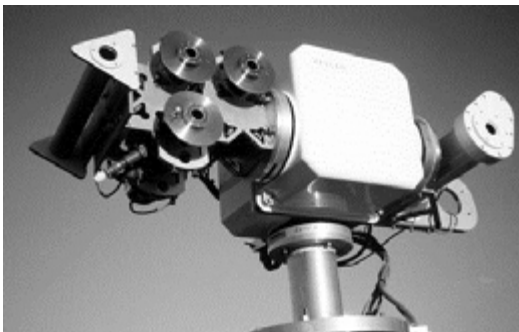
Fig. 3.1 Pyrheliometers for measuring direct-normal solar radiation.
