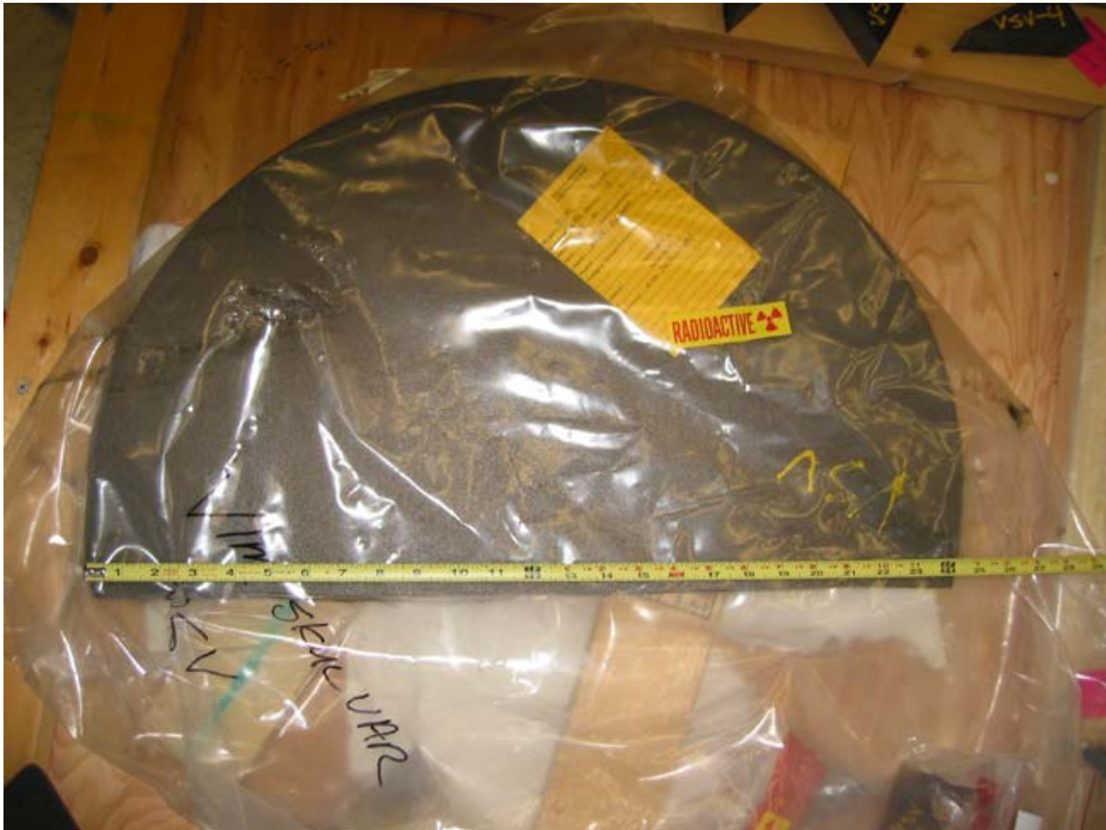
Figure 2: A remnant of the original U-6Nb VSV plate measuring approximately 2 feet in diameter. An outside edge from this lot was used to manufacture a cube.
