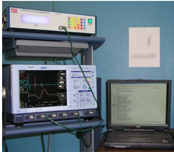
Figure 6: The instrumentation used to make the ultrasonic time-of-flight measurements includes a Panametrics 5800 pulser/receiver, LeCroy 950 wavepro oscilloscope, and a notebook computer.
