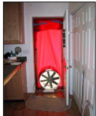
Figure 7. Blower door installed in the Hathaway House
