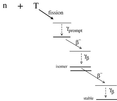
Figure 1: Illustration of some processes leading to the production of post-fission  $\beta$ -delayed photons. Here  $\gamma_{prompt}$  represents the photons emitted by the highly excited fragment nucleus born just after fission. Beta-delayed photons represented by the source function  $s_\gamma$  described in the text are labeled  $\gamma_\beta$ .
