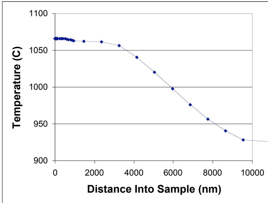
Figure 1.4 – Temperature profile versus distance into the sample for a time snapshot at 500 ns.
