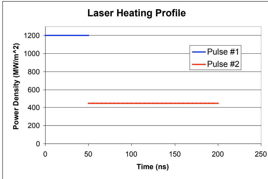
Figure 1.2 – Heating profile for the two laser pulses.
