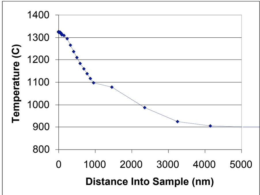
Figure 1.3 – Temperature versus distance profile for the time at which the largest surface temperature is observed. Snapshot is taken at 50 ns after the laser pulse was initially turned on.
