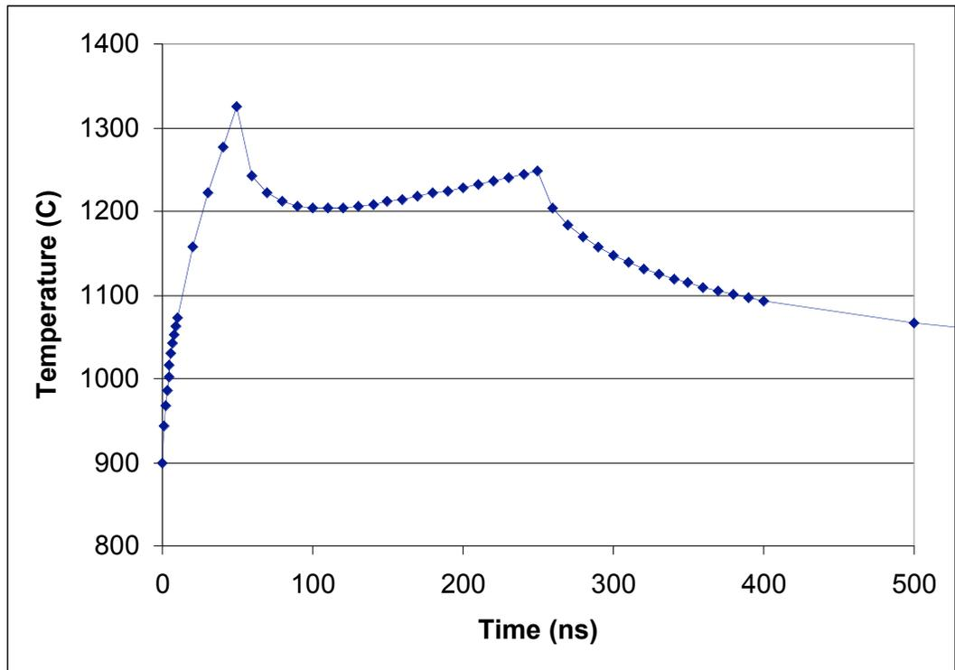
Figure 1.1 - Time-temperature history for surface of potassium-doped aluminosilicate.
