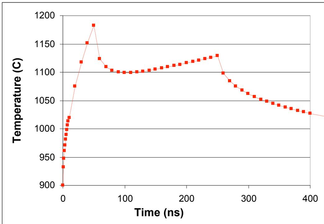
Figure 1.5 – Temperature versus time history of the ceramic surface with a thermal conductivity of the ceramic set to 7 W/m-K.
