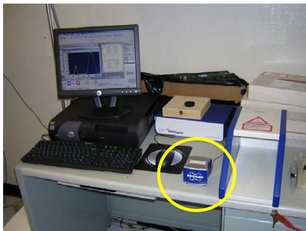
Figure 9. The NMR MOUSE. Polymeric materials are placed on MOUSE (outlined) and scanned via low field spin-echo relaxometry methods discussed in test.
