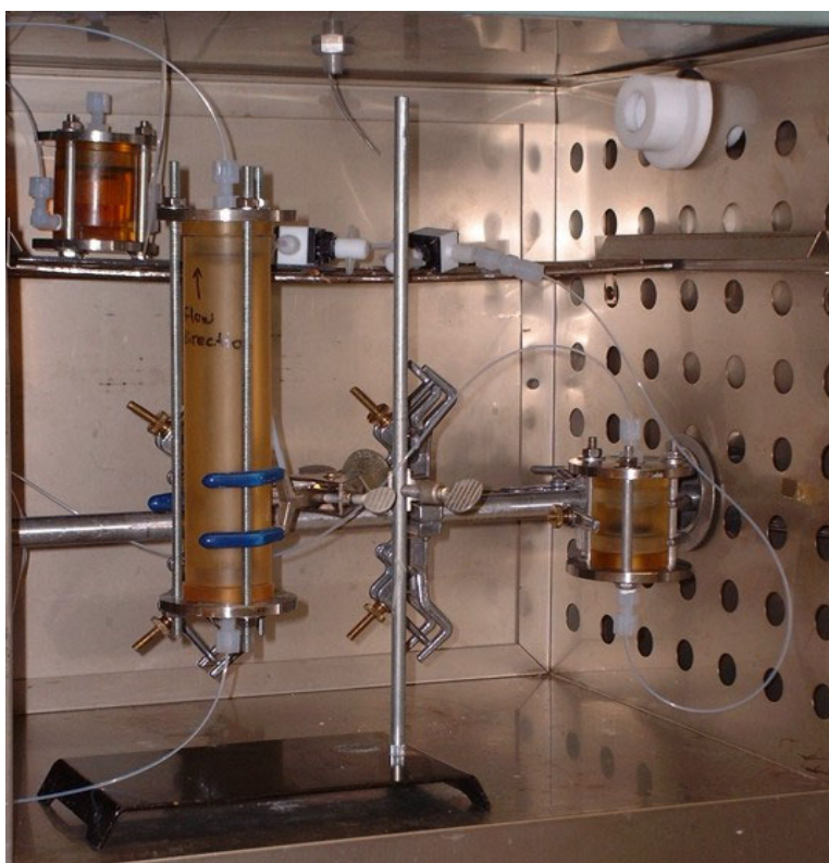
Figure 6. Glass dissolution experimental set-up showing flow-through cell attached to shaker arm at right, pre-reactor cell at left and bubbler cell at upper left.
