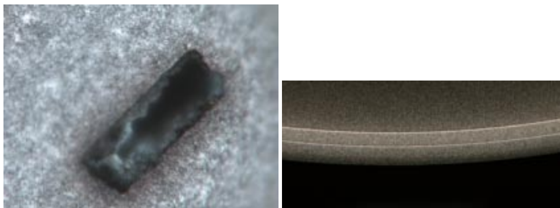
Figure 2. Left, an image of the big hole drilled in the first capsule tested. Right, a radiographic image of a portion of the shell wall before heating, clearly showing the outer Be and inner plastic layers.
