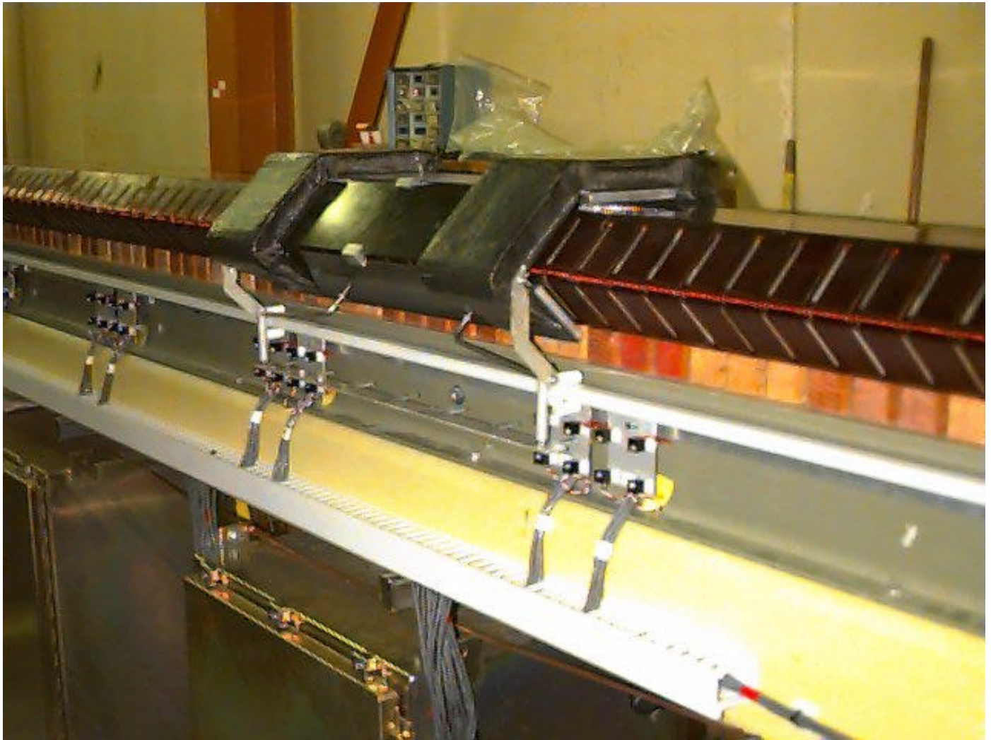
Figure 9. Close-up of the cradle, sensors, and comb that blocks the sensor signals in order to initiate the drive pulse as the cradle moves down the track.
