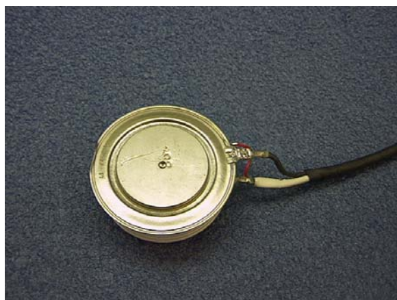
Figure 2. Photograph of the SDM170HK MOS Turn-Off Thyristor fabricated by Silicon Power Corporation.
