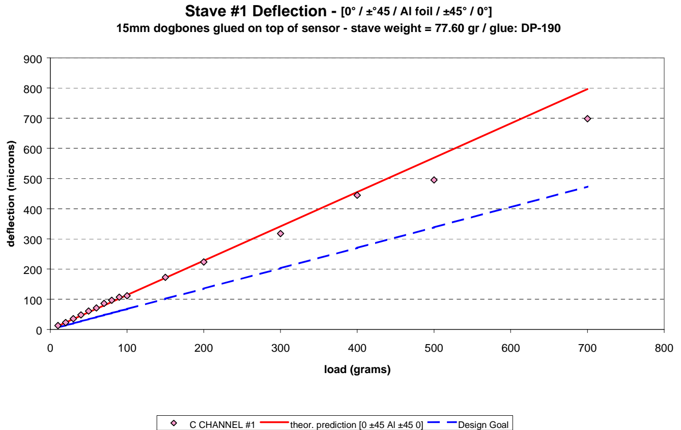
Figure 8 – Stave #1 mockup deflection study. The 15 mm wide dog-bones (wirebonds protections) are glued on top of the silicon sensors. The C channel structural elements are ~13.2mm wide \times ~9.0mm tall and made of carbon fiber prepreg (Mitsubishi K139, [0^\circ, \pm 45^\circ] lay-up) with interposed a 1 mil aluminum sheet. The core is made of Rohacell, 200 \mu m thick carbon skin and 50 \mu m thick Kapton.
