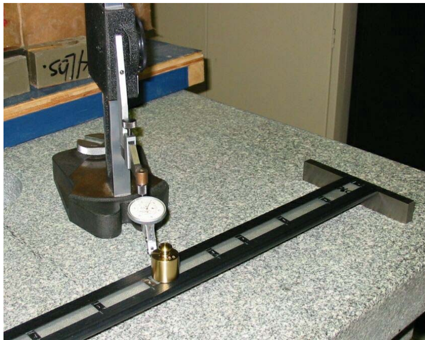
Figure 6 – Setup of the deflection test.
