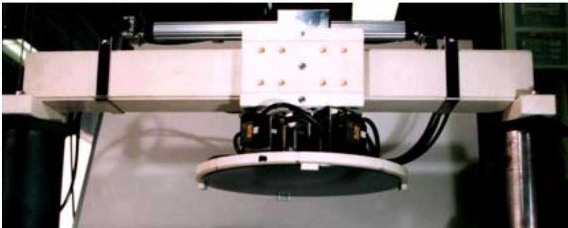
**Figure 12: Electrostatic Wafer Levitation Device**
