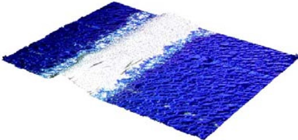
**Figure 16: Hot melt material shown after firing using the 3D model capabilities of the Syncroscopy system**
