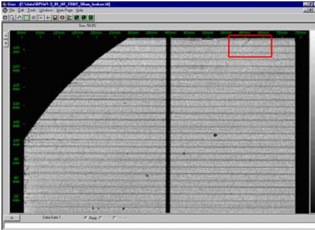
**Figure 26: SAM image of the initial crack on the wafer captured in the red box**
