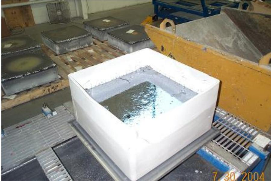
**Figure 7: Clean, Shiny Ingot Surface from Experimental Cover**
