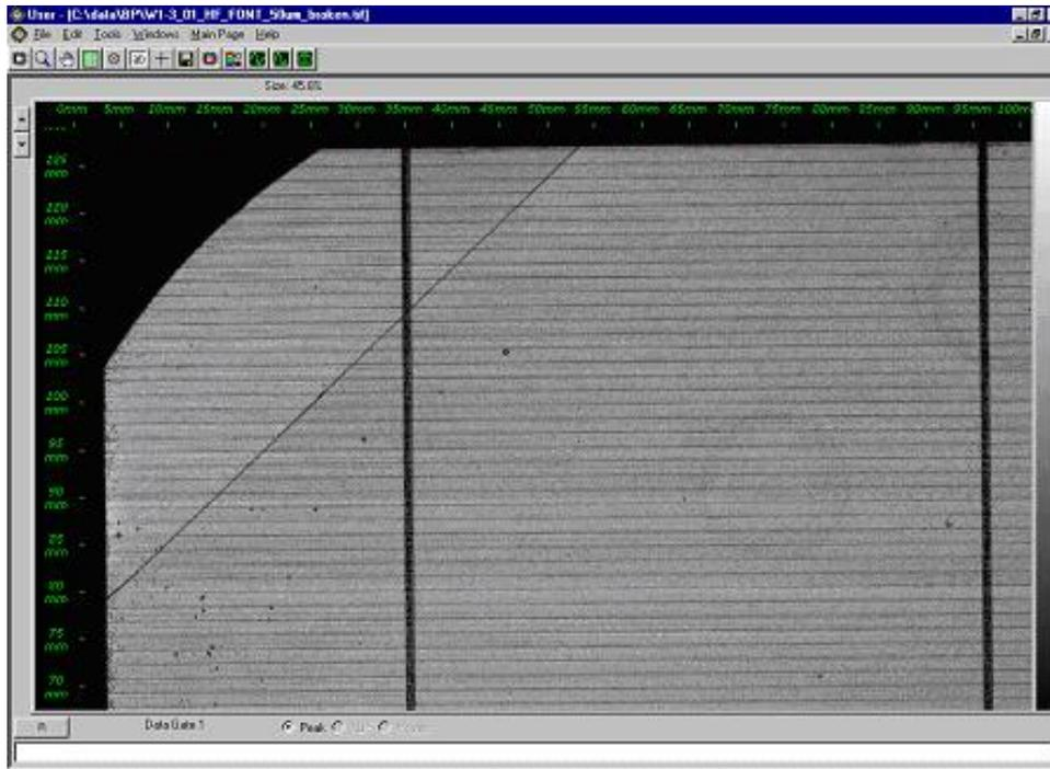
**Figure 27: SAM image of the same area of the wafer as Figure 26 after stress. The initial crack had propagated across the wafer’s corner causing it to break.**
