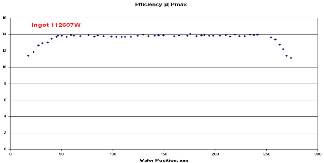
**Figure 4: Cell Efficiency as a Function of Position in Large Ingot**
