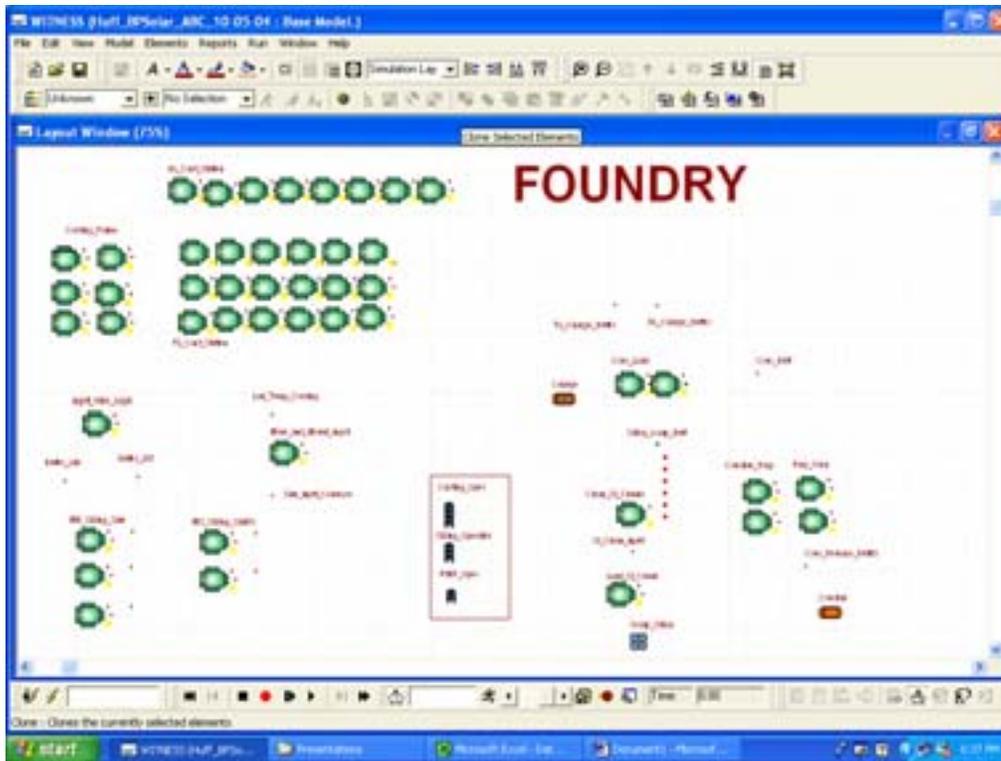
**Figure 30: A section of the discrete-event simulation model depicting foundry operations**
