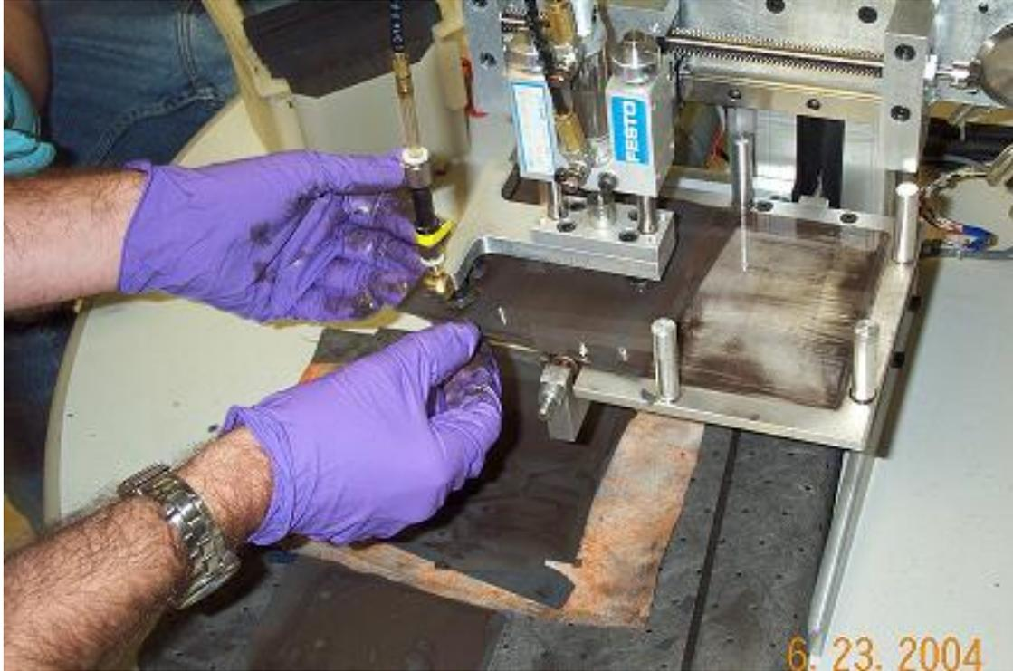
**Figure 11: ARRI Wet Wafer Singulation Prototype in Operation**
