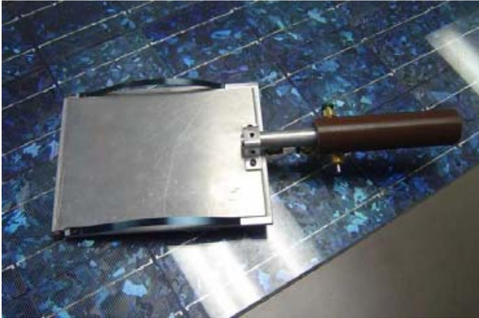
**Figure 14: Airjet Pickup Tool**
