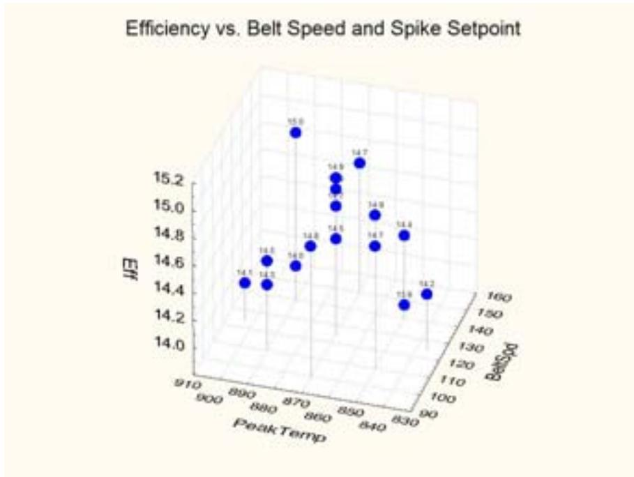
**Figure 17: Cell Efficiency versus 3 Variables from RSM Trial of Hot Melt Paste Firing Conditions**
