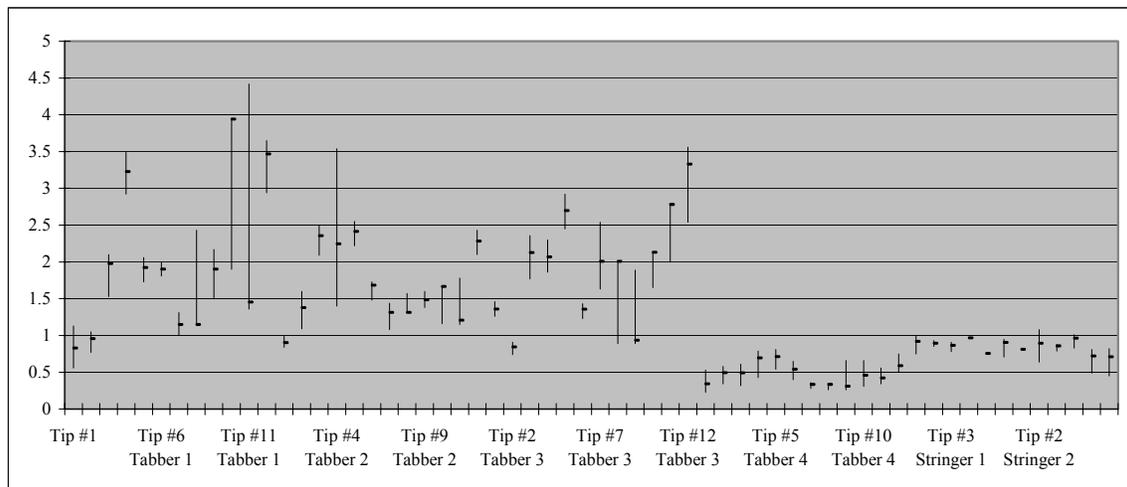
**Figure 24: Force Applied by Hot Bar Tip While Making a Solder Bond**
