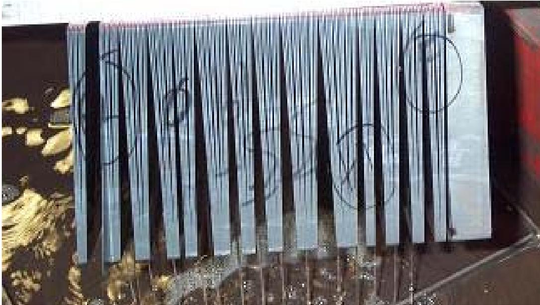
**Figure 8: Thin Wafer Comb as it came off of the Wire Saw**
