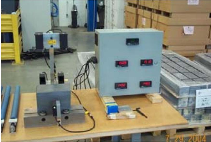
**Figure 29: Brick Measurement System**
