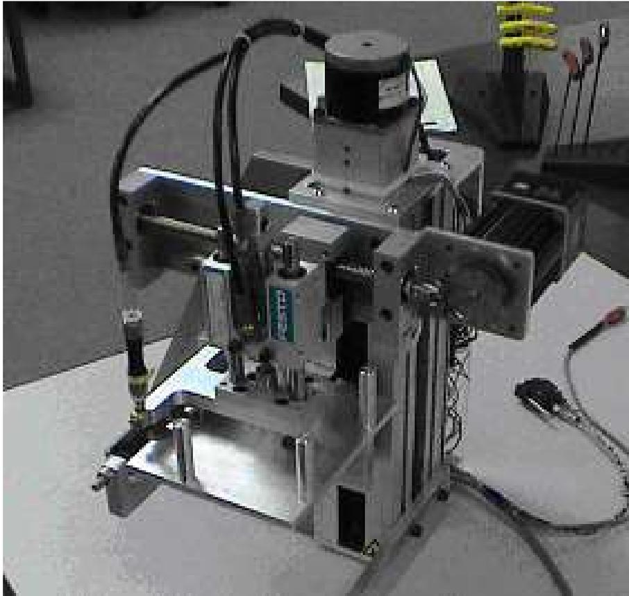
**Figure 10: ARRI Wet Wafer Demounting Prototype**
