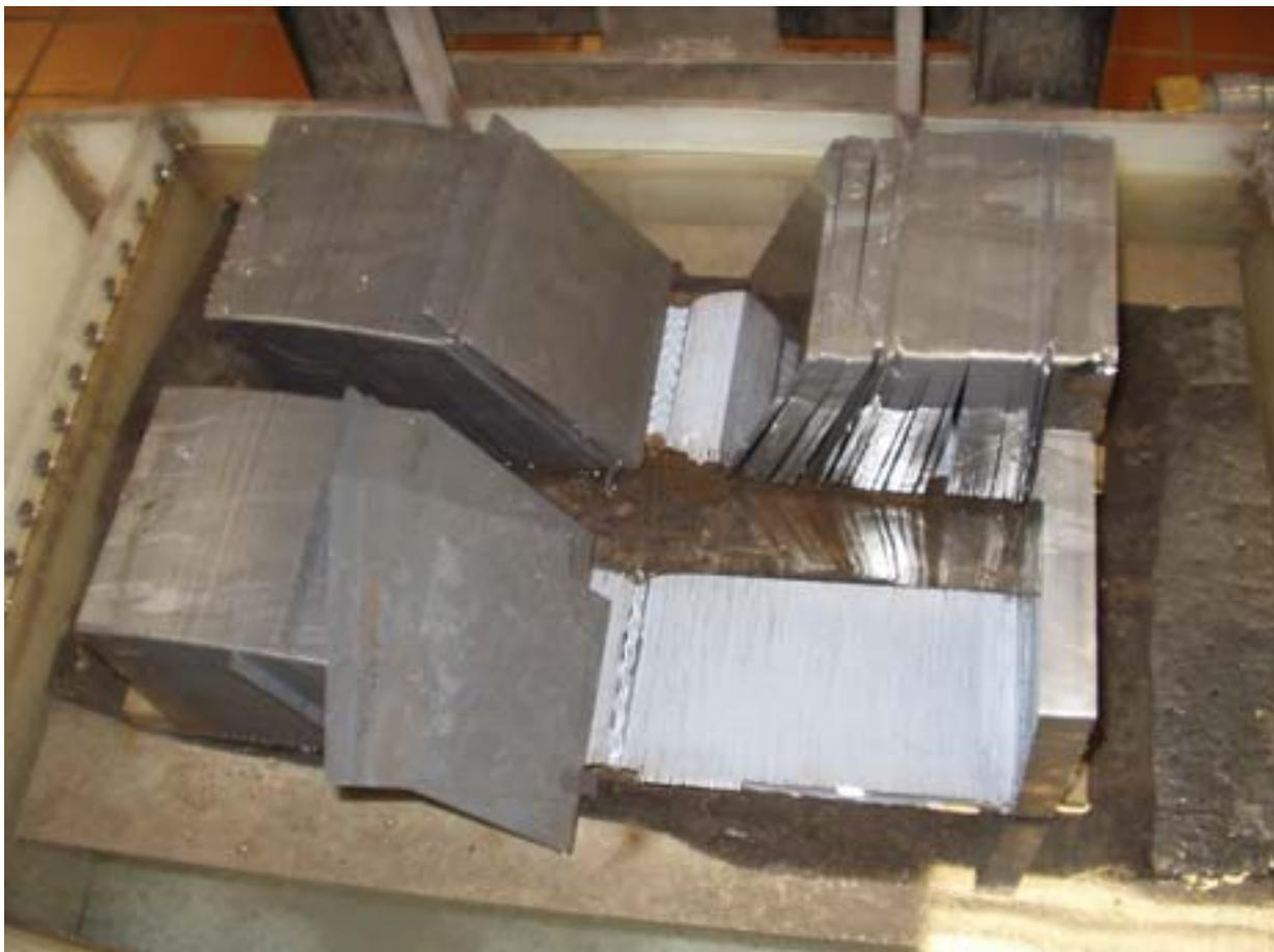
**Figure 9: Blue Glue trial – Glue releases from the wafer not the mounting beam**
