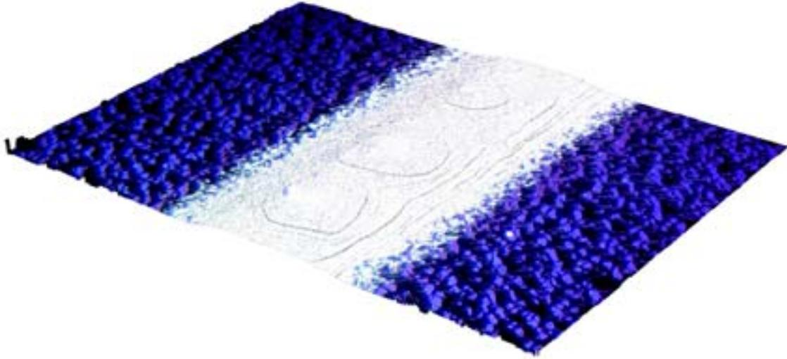
**Figure 15: Standard paste deposition shown after firing using the 3D capabilities of the Syncroscopy system**
