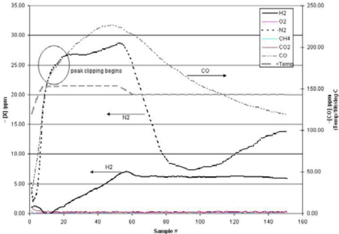
**Figure 6: Concentration of Impurities during Casting Run**
