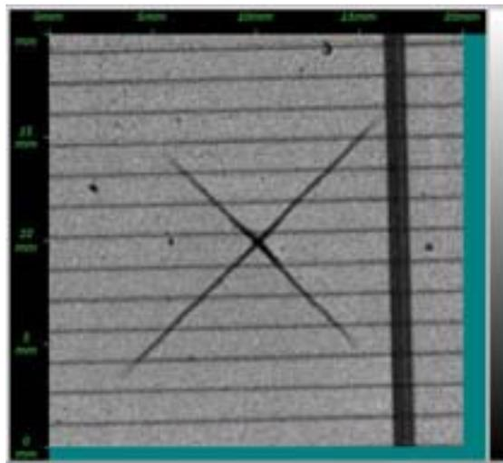
**Figure 28: SAM image of STAR crack**
