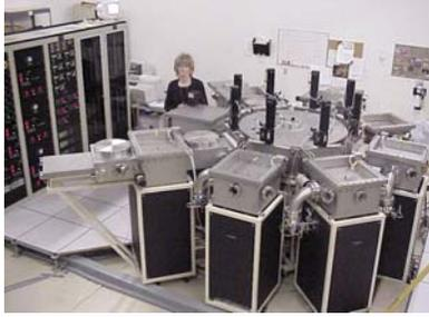
**Figure 15:** large area sluter tool with multiple PECVD and sputtering chambers. Substrate size: 30cmx40cm.
