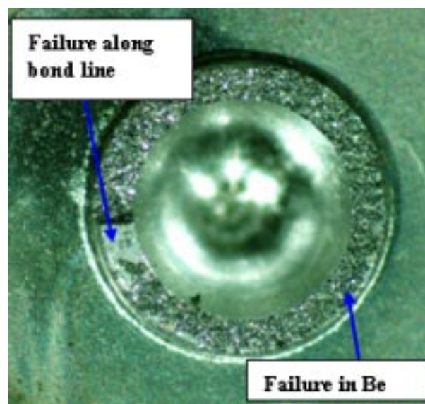
Figure 7. Optical photograph of failure of a Be-Be bond. Approximately 80% of the bond failed in the beryllium metal, indicating that most of the bond was as strong or stronger than the beryllium metal.
