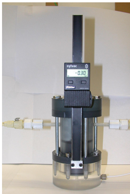
Figure4B. Photograph of the Shrinkage Coefficient Measurement Cell
