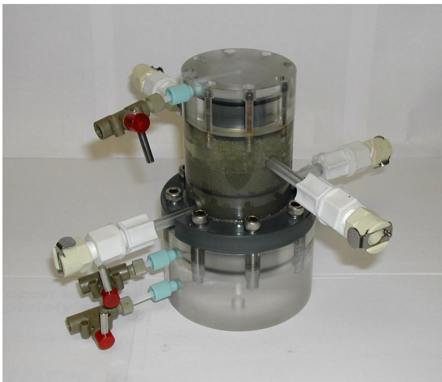
Figure5B. Photograph of the Crack Propagation and Imaging Cell
