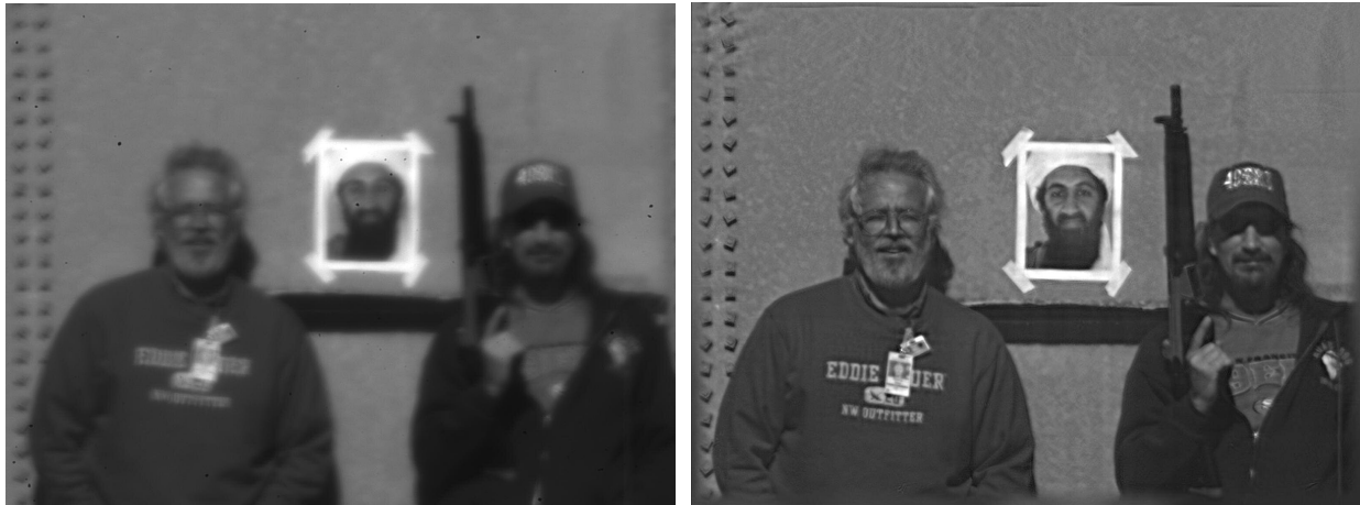
(a) Blurry, unprocessed image (b) Enhanced image from 40 raw frames
