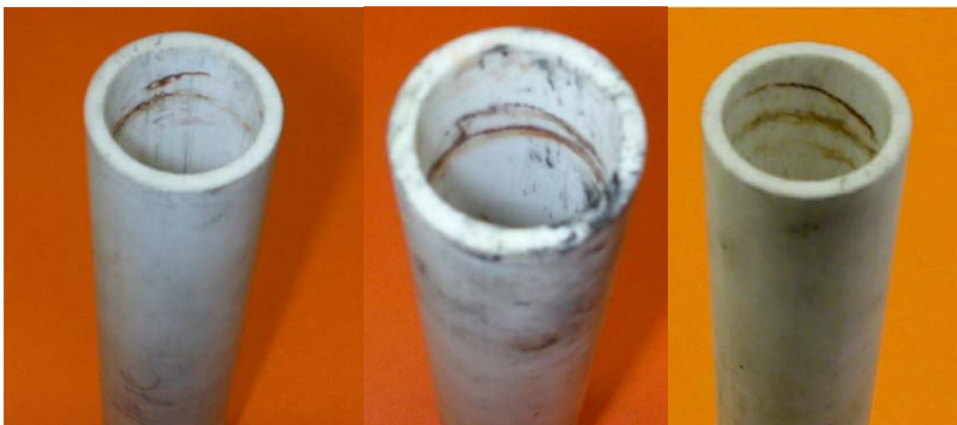
Fig. 2. Three photographs are shown of nominally vertical cells of inside diameter, 2 cm (roughly 3 cm 2 working area), showing that the orientation of the electrode assembly (indicated by corrosion marks on the cells) were not controlled and generally were not strictly horizontal. Tilting the cell by an angle large compared with the angle of the electrode assembly (relative to horizontal) led to a substantial deviation from horizontal.
