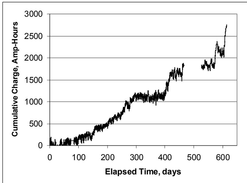
Figure 6.8. Battery charge-discharge history, showing overcharging
