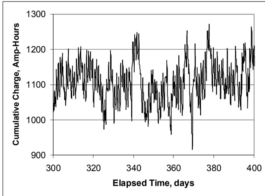
**Figure 6.9. Period of battery history showing no overcharging**
