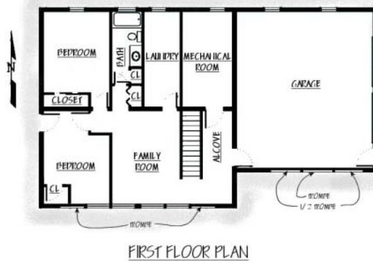
**Figure 3.4. The first floor plan of the Van Geet home, as built**
