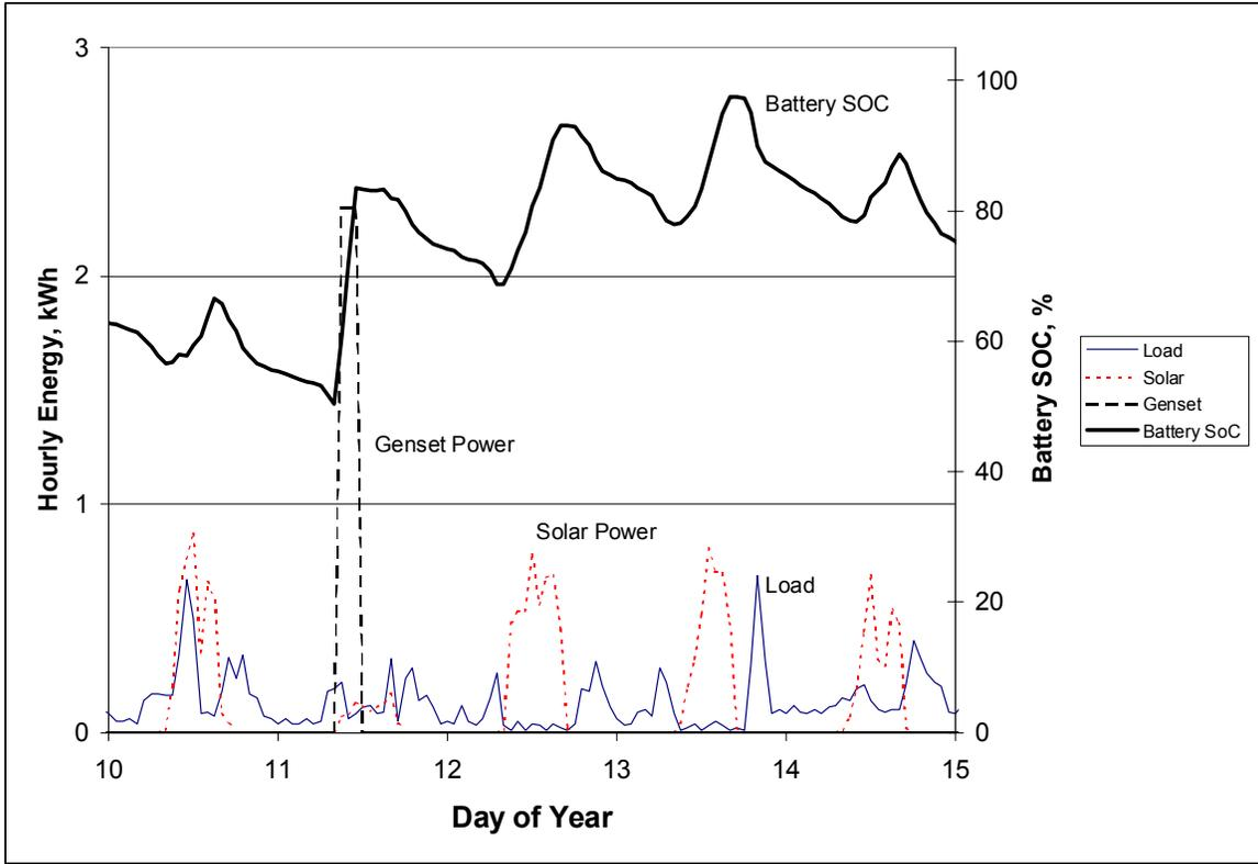
**Figure 6.13. Modeled hourly performance of the electrical system**
