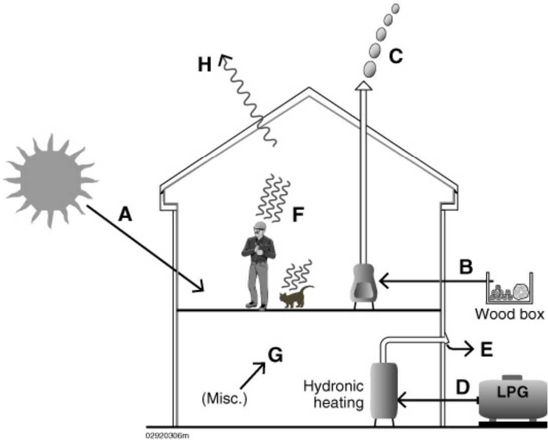
Figure 4.1. Pictorial diagram of thermal energy flows in and out of the house
