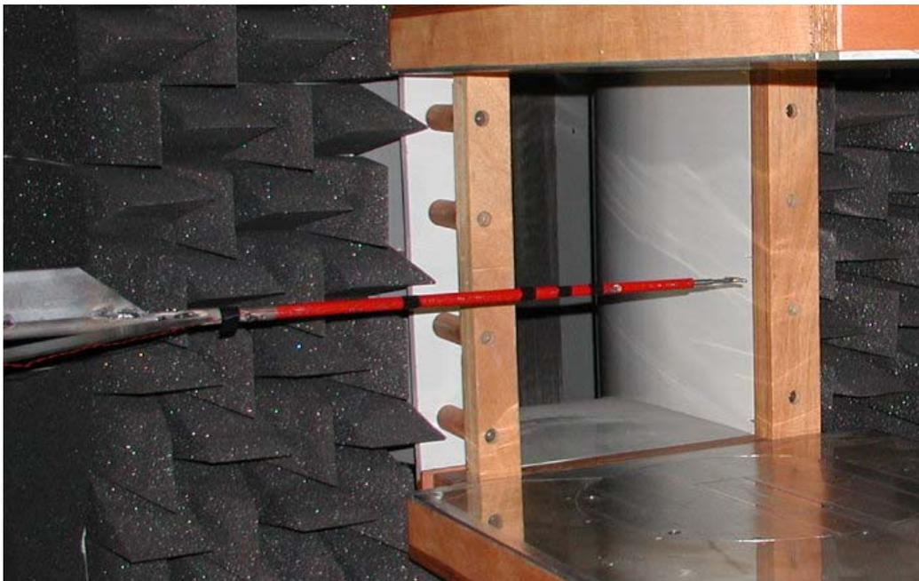
**Figure 5. Hot-wire probe in empty test section**
