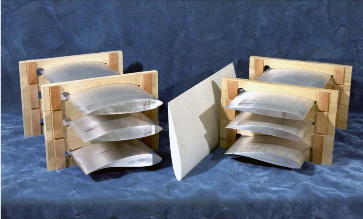
**Figure 7. Photograph of tested airfoil models (NACA 0012 model in white)**
