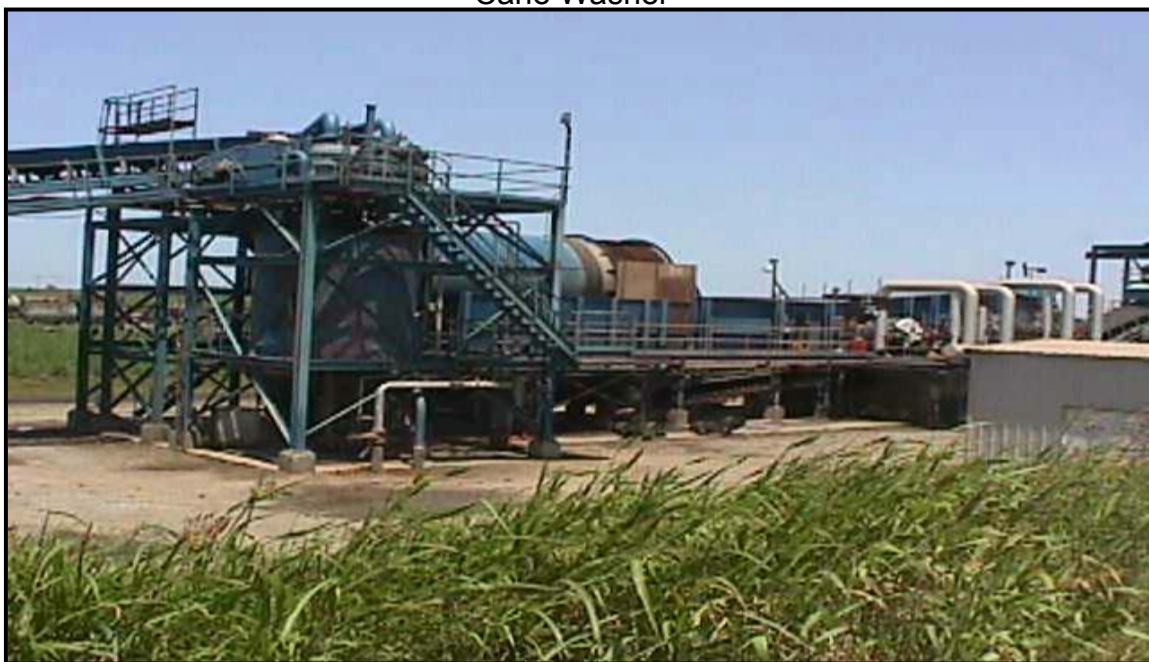
Figure 11 Cane Washer
