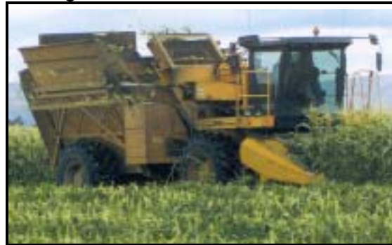
Figure 6, Ear Corn Harvester
