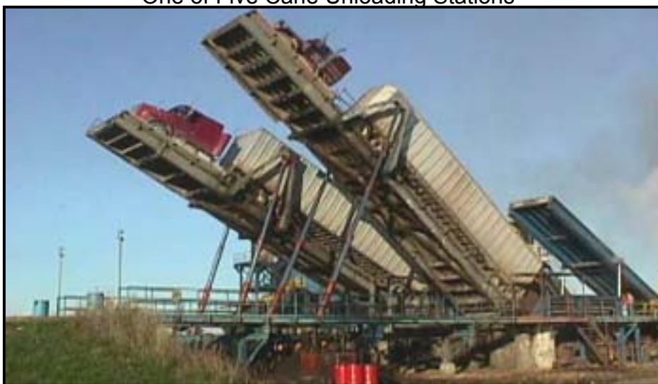
Figure 7 One of Five Cane Unloading Stations
