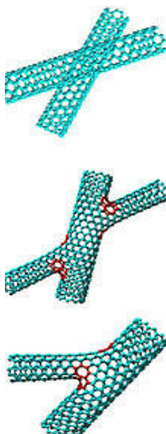
Figure 3. Welding SWNTs at different sites
