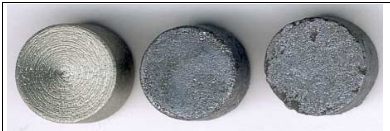
Fig. 5. Images of the Mo batches prior to (1) and after corrosion tests in a phosphate (2) and ultraphosphate (3) glass.
