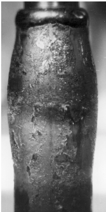
Fig. 2. Appearance of fuel rod near top end.
