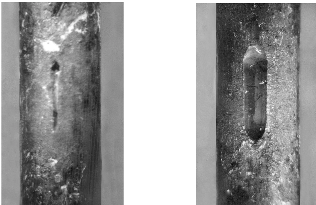
Fig. 1. Appearance of fuel rods under spacer grids.
