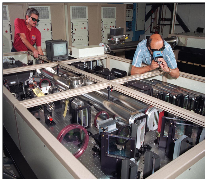
Figure 1. LLNL's laser peening system.
