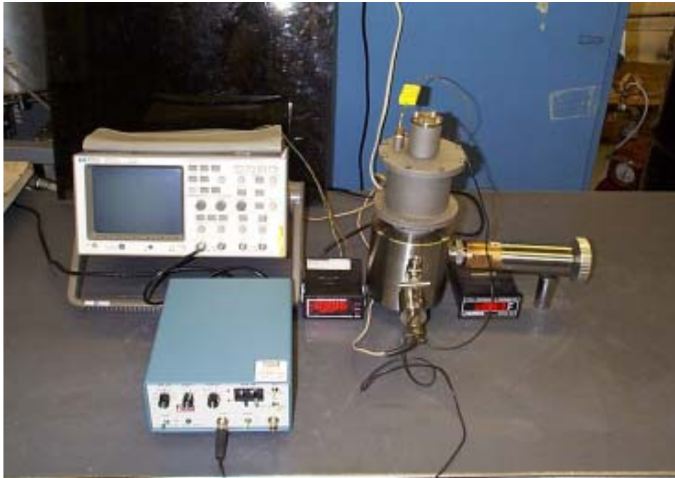
Figure 4. Experimental apparatus for ultrasound measurements.
