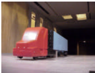
Figure 1. Generic Conventional Model (GCM) in wind tunnel.
