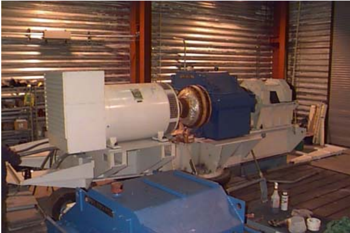
Figure 6 – Original synchronous generator and fluid coupling
