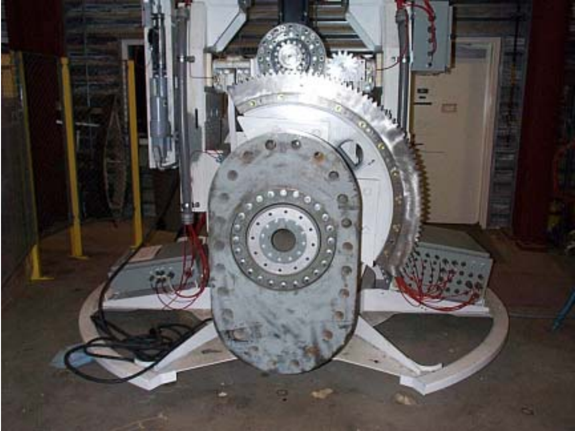
Figure 5 - CART hub with new electromechanical pitch system
