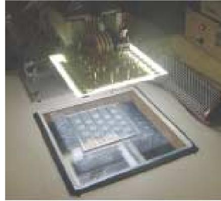
Figure 4.1. Cell IV system with 18-pogo-probe contacting head and pneumatic actuation
