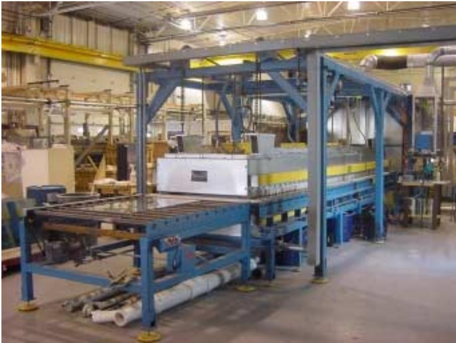
Figure 3.2. APCVD system for module-scale buffer-layer deposition.
