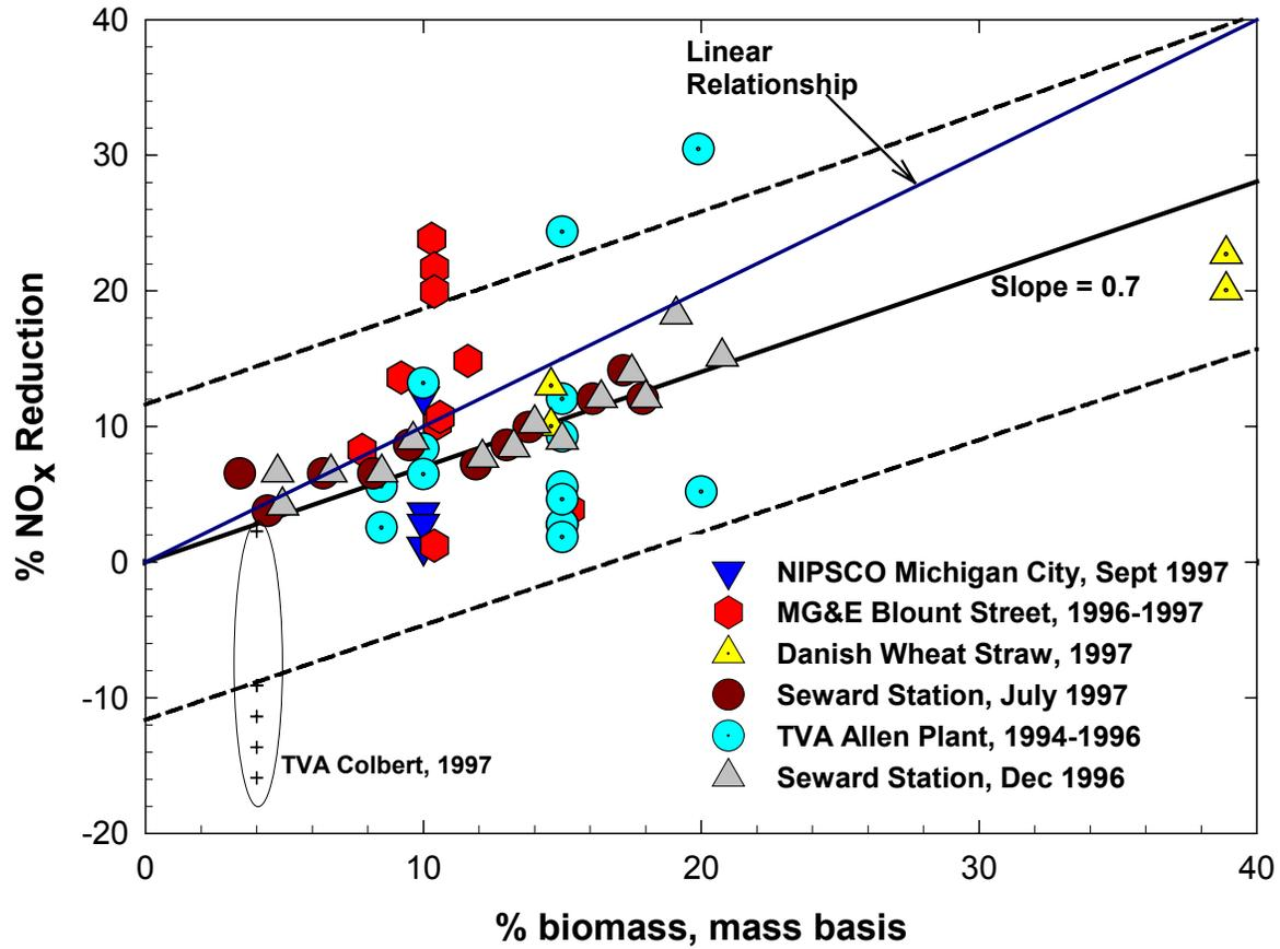
**Figure 1:** A summary of NO<sub>x</sub> reduction from a number of biomass/coal cofiring full-scale and pilot-scale demonstration tests, based on the mass input of biomass. Dashed lines are 95% prediction limits that encompass the range of variability in the measured data.
