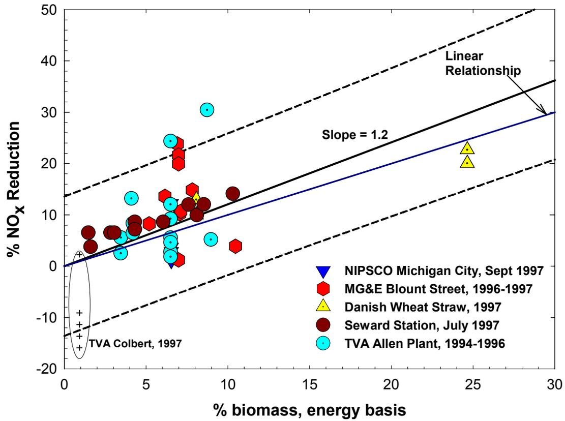
**Figure 2:** A summary of NO<sub>x</sub> reduction from a number of biomass/coal cofiring full-scale and pilot-scale demonstration tests, based on the energy input of biomass. Dashed lines are 95% prediction limits that encompass the range of variability in the measured data.
