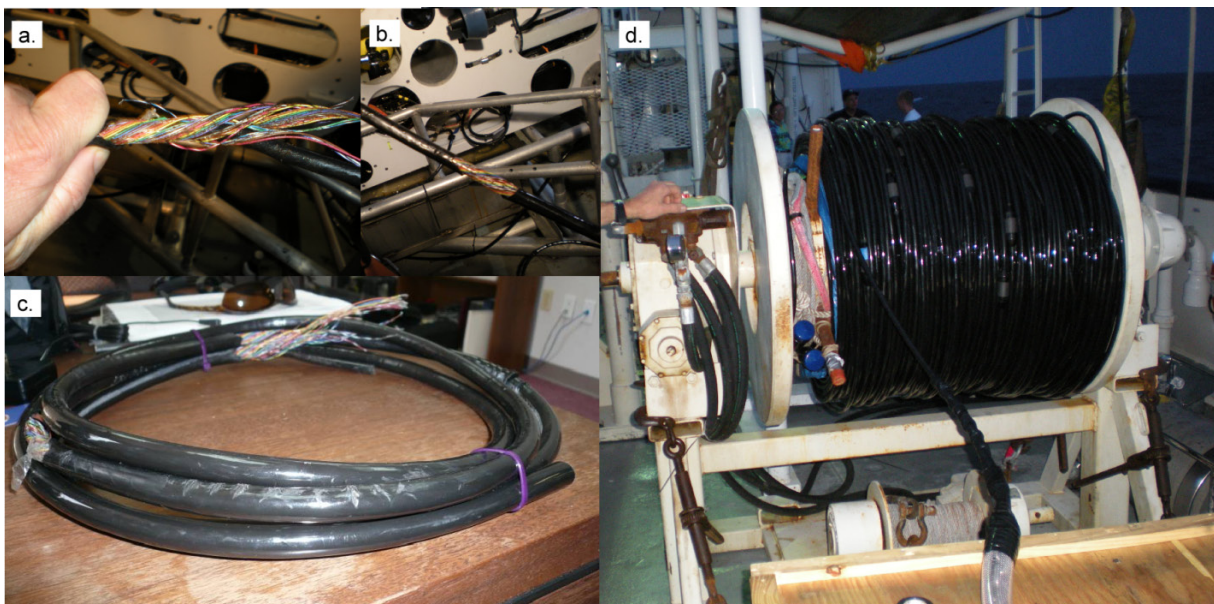
Figure 2.2 Seafloor electrode arrays. a. The first array was 540-m long, with 28-electrode array spaced 20 m apart. During the first deployment the array was apparently bitten by sharks, leaving only 8 of the original 28 electrodes attached to the ROV. b. Section of missing cable jacket of the 540-m array after the system was retrieved in June 2008. c. Retrieved array segment 540-m array showing triangular bite marks in the cable jacket. d. Replacement, 1100-m, 56-electrode array spooled on a winch and ready for deployment in June 2009. A length of heavy chain in a clear plastic tube is connected to the tail-end of the array in the foreground, to insure the array sinks rapidly to the bottom to avoid shark damage.
