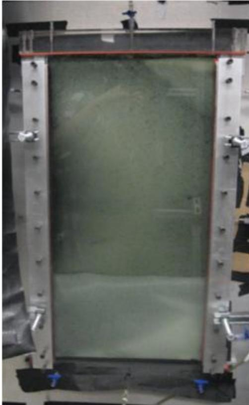
**Figure 2.1. Test chamber filled with F110 sand (bottom) and F30 sand (top).**
