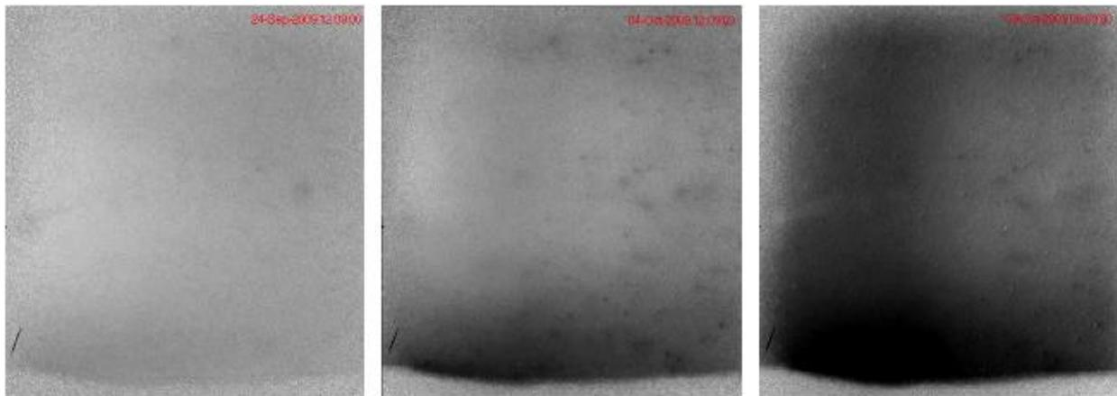
**Figure 2.3.** Time sequence images spanning 16 days (left to right) of the KB-1 + CFDA flow-through experiment, with emitted light indicated by gray shading and suspected biofilm formation indicated by darken regions.
