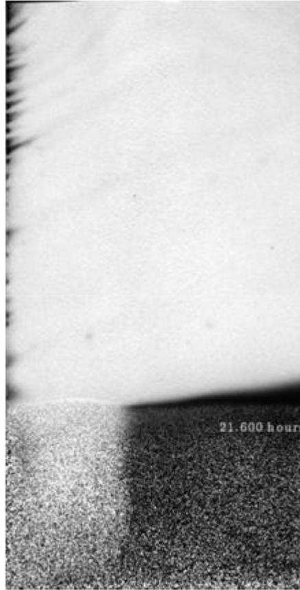
**Figure 2.2.** Left-to-right flow of de-ionized water displacing dyed water from the chamber.
