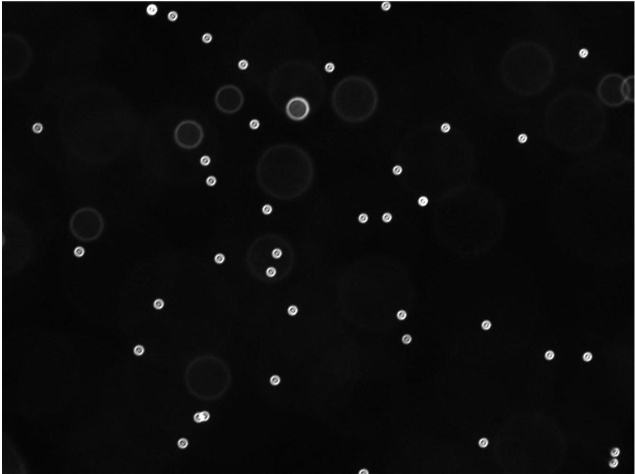
**Figure 1.1. Photomicrograph of fluorescent microspheres used to test and calibrate imaging methodology (630X magnification, with FITC filter).**
