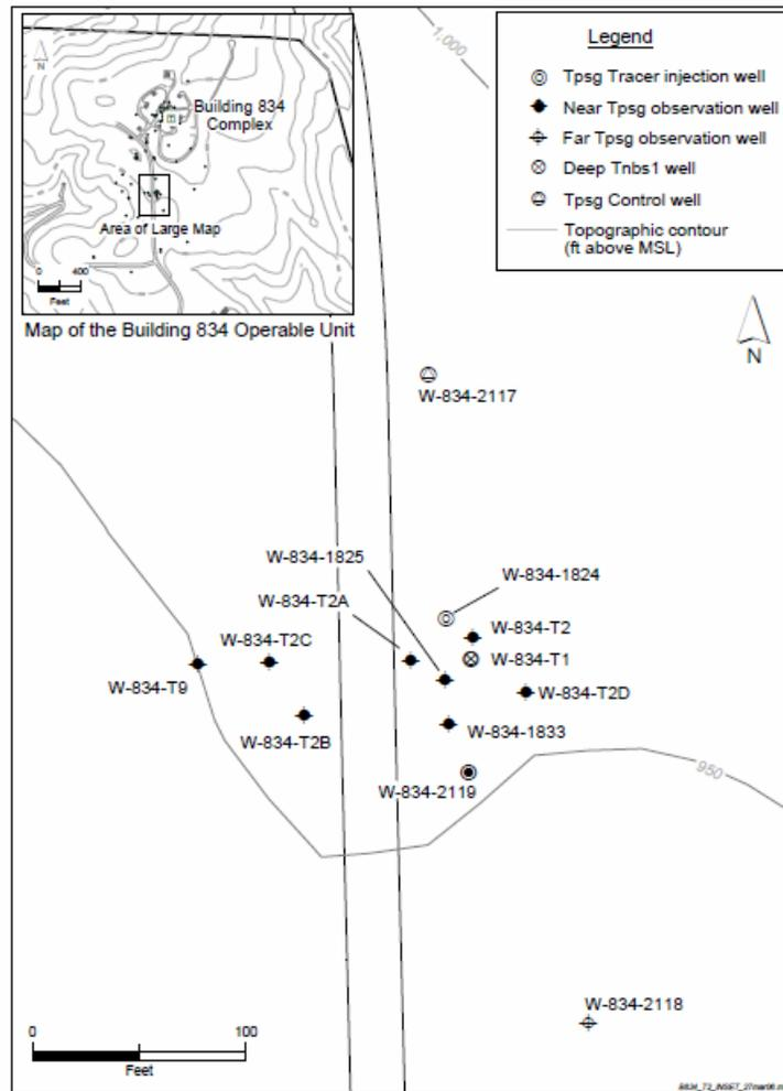
Figure 3.1. Map of the B834/T2 area at Site 300, indicating locations and types of wells used in the bioaugmentation treatability test.
