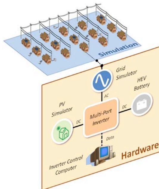
*An HIL simulation at NREL will enable evaluation of complex scenarios and testing of second-use batteries in real-world conditions, without risking damage to utility hardware or interruption of service.*
