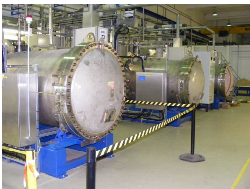
Figure 44. UK block test stand configuration with single block
