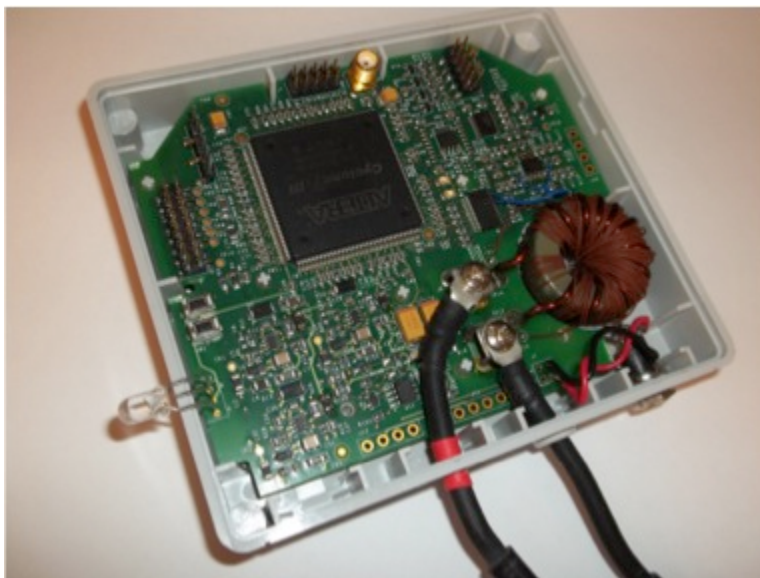
Figure 8. Prototype arc fault detector circuit
