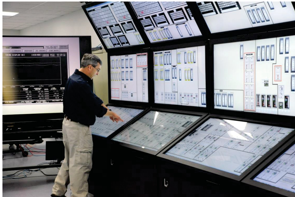
Figure 4. HSSL used to evaluate digital upgrades in a hybrid control room
