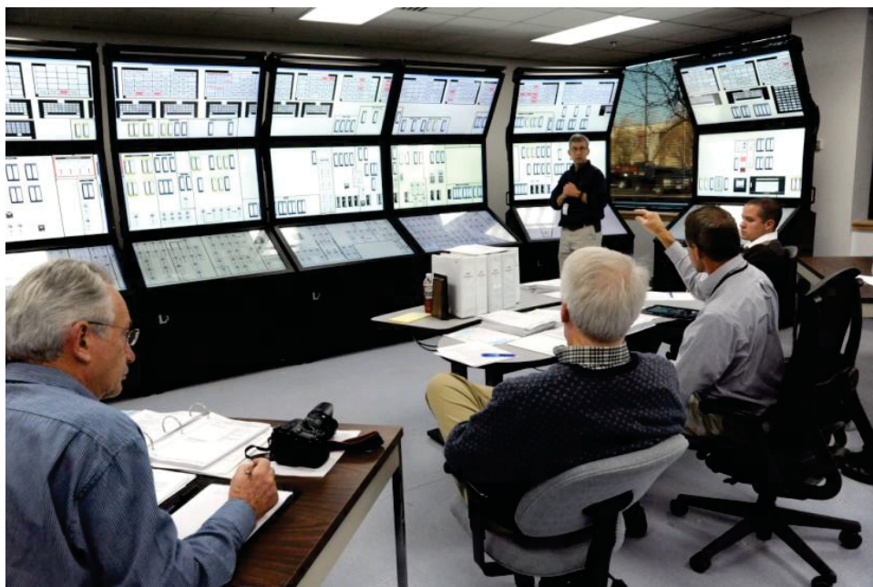
Figure 5. HSSL being used for control room operator studies on control room function allocation
