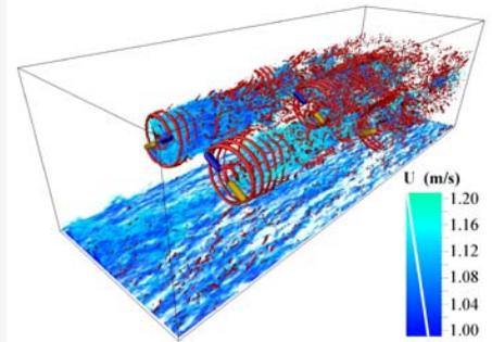
Current turbine array simulation using LES model. Illustration by Mathew Churchfield, NREL
