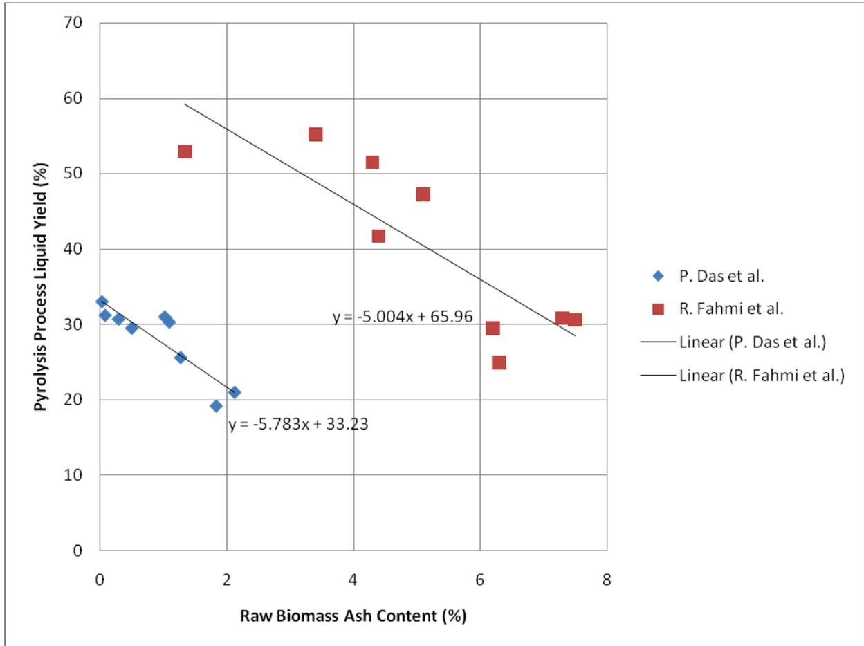
**Figure 4: Pyrolysis process yield as a function of feedstock ash content.**
