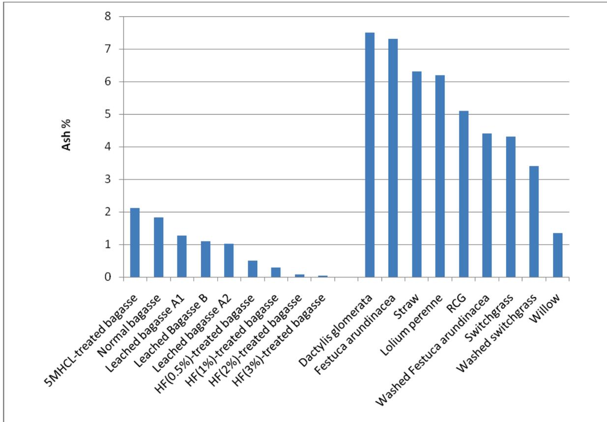
Figure 5: Ash % as a function of biomass type and wet separation operation.
