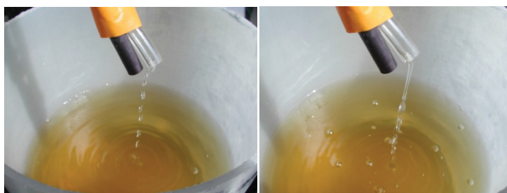
Figure 8. Nitrogen backflow before (left) and after (right) backflush.
