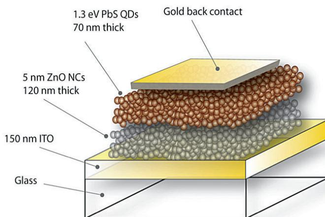
In 2011, NREL researchers certified the first all-quantum-dot solar cell, which combines a 70-nanometer-thick layer of lead sulfide quantum dots (QDs) with a 150-nanometer-thick layer of zinc oxide nanocrystals (NCs). Current is collected from the transparent conductive oxide layer, formed from indium tin oxide (ITO), and the gold back contact. The top of the solar cell, shown face down in this illustration, is protected with a layer of glass.
