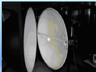
62" integrating sphere for photometric testing
