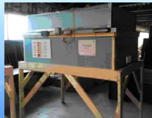
Lamps run continuously on a 3-hour on, 20-minute off cycle at 45°C inside of temperature control chambers
