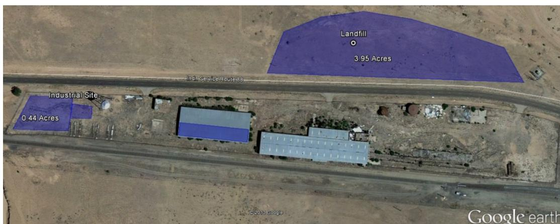
**Figure 6. Aerial view of the feasible areas for PV at the Santo Domingo Pueblo industrial site (ground-mounted in dark blue and roof-mounted in light blue)**
