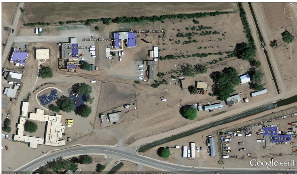
**Figure 7. Aerial view of the feasible areas for PV within the Santo Domingo Pueblo (no ground-mounted PV potential exists; existing municipal buildings with potential roof-mounted PV in blue)**
